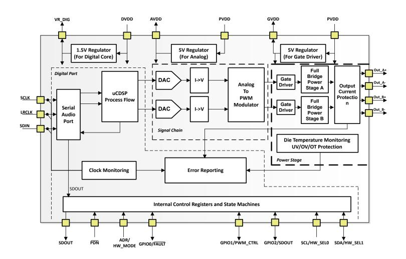
Figure 6-1. Functional Block Diagram
