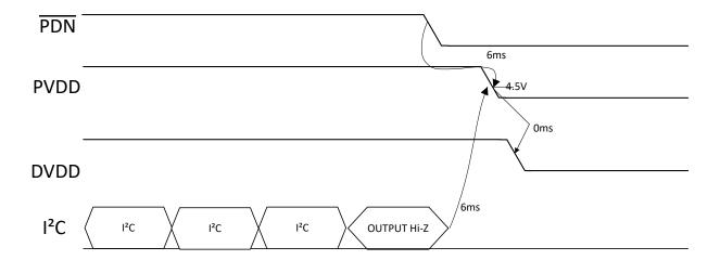
Before PVDD/DVDD power down, Class D Output driver needs to be disabled by PDN or by  $I^2C$ . At least 6ms delay needed based on LRCLK(Fs) = 48kHz, digital volume ramp down update every sample period, decreased by 0.5dB for each update, digital volume = 24dB. Change the value of register 0x4C and 0x4E or change LRCLK rate, the delay changes.
