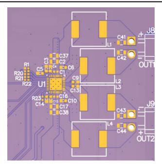
Figure 7-4. 2.0 (Stereo BTL) Top Copper View
