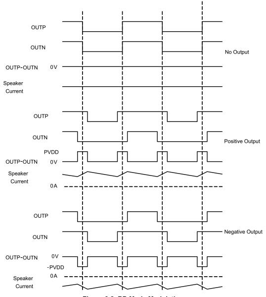
Figure 6-8. BD Mode Modulation
