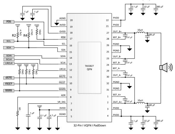
Figure 7-2. Sub-woofer (PBTL) Application Schematic
