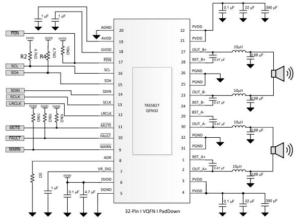
Figure 7-1. 2.0 (Stereo BTL) System Application Schematic
