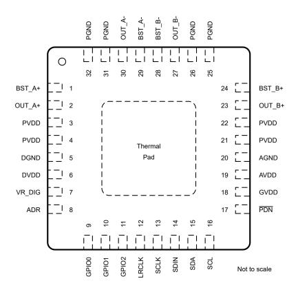
Figure 4-1. RHB (VQFN) Package, 32-Pin PadDown, Software Mode, Top View
