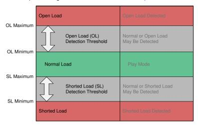
Figure 9-6. DC Load Diagnostic Reporting Thresholds
