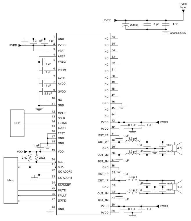
Figure 10-2. Typical 2-Channel BTL Application Schematic
