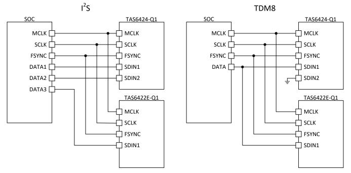
Figure 9-1. Digital-Audio Data Connection
