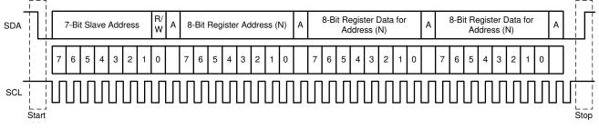
Figure 9-9. Typical I<sup>2</sup>C Sequence
