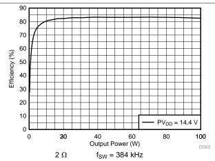
Figure 13. PVDD Power Efficiency vs Total Output Power
