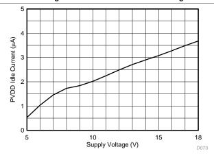
Figure 18. PVDD Standby Current vs Voltage
