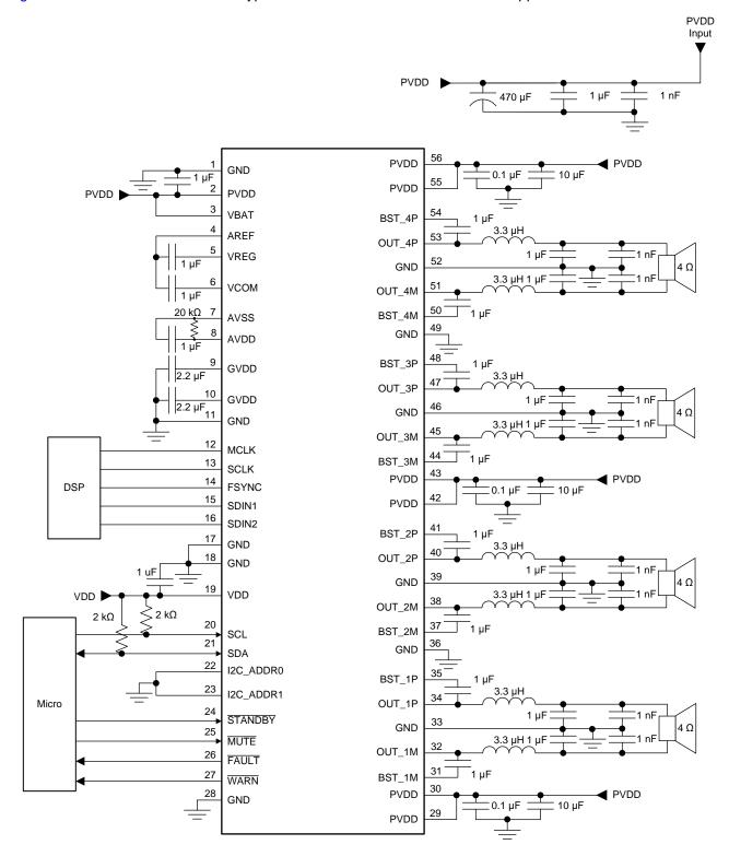
Figure 79. TAS6424M-Q1 Typical 4-Channel BTL Application Schematic
