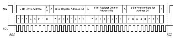
Figure 41. Typical I<sup>2</sup>C Sequence
