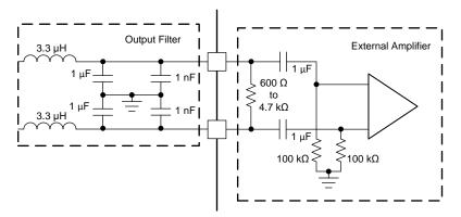
Figure 78. External Amplifier Input Configuration for Line Driver
