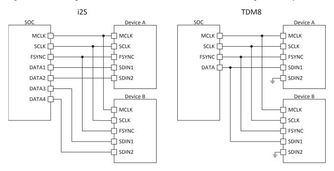
Figure 31. Digital-Audio Data Connection
