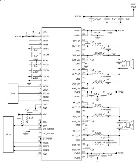
Figure 82. TAS6424M-Q1 Typical 2-Channel PBTL Application Schematic
