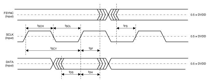
Figure 32. Serial Audio Timing
