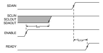
Figure 6-2. Timing for t<sub>STOP</sub>
