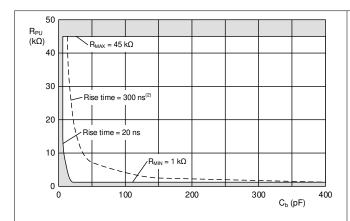
Figure 8-4. Example Bus Requirements for 3.3 V Systems
