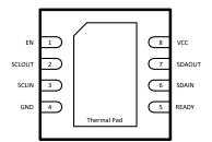
Figure 4-2. 8-Pin WSON, DRG Package (Top View)
