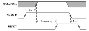
Figure 6-1. Timing for  $t_{\text{EN}},\,t_{\text{IDLE}(\text{READY})},$  and  $t_{\text{DIS}}$
