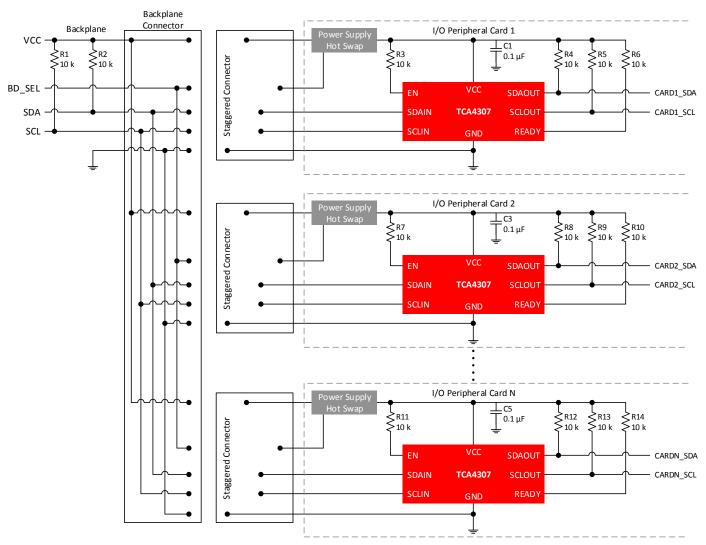
Figure 8-6. Backplane Application Schematic
