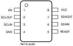
Figure 4-1. 8-Pin VSSOP, DGK Package (Top View)
