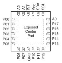
The exposed center pad, if used, must be connected as a secondary ground or left electrically open.
