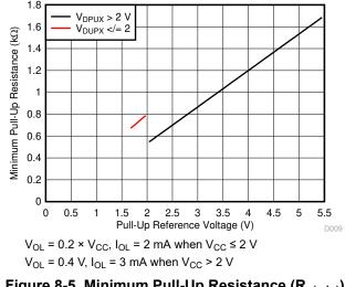
Figure 8-5. Minimum Pull-Up Resistance ( $R_{p(min)}$ ) vs Pull-Up Reference Voltage ( $V_{CC}$ )
