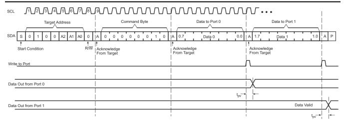
Figure 7-7. Write to Output Port Registers
