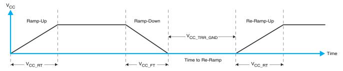
Figure 9-1. V<sub>CC</sub> Is Lowered Below 0.2 V Or 0 V And Then Ramped Up To V<sub>CC</sub>
