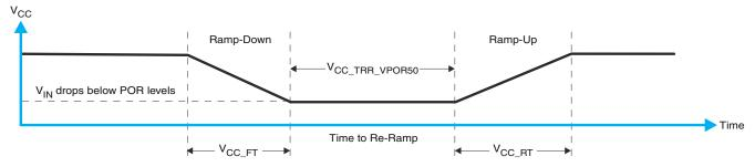
Figure 9-2.  $V_{CC}$  Is Lowered Below The Por Threshold, Then Ramped Back Up To  $V_{CC}$
