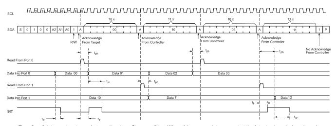
Figure 7-9. Read Input Port Register, Scenario 1
