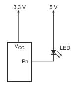
Figure 8-3. Device Supplied by Lower Voltage
