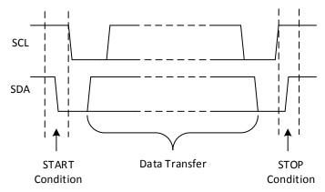
Figure 7-3. Definition of Start and Stop Conditions
