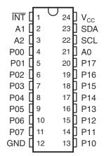
Figure 5-1. DB, PW (TSSOP) Package 24-Pin (Top View)
