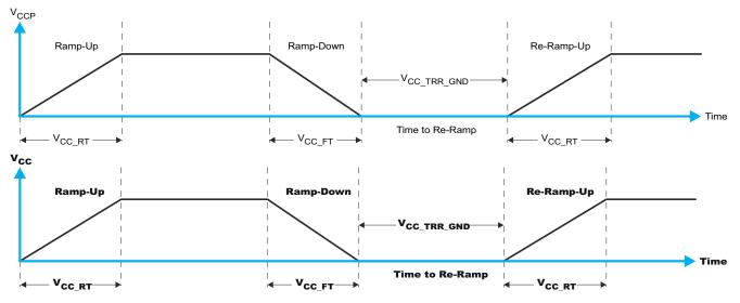
Figure 8-6. V<sub>CCP</sub> is lowered below 0.2 V or 0 V and then ramped up
