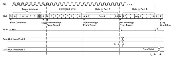
Figure 7-9. Write to Output Port Register
