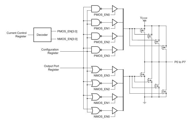
Figure 7-3. Simplified output stage
