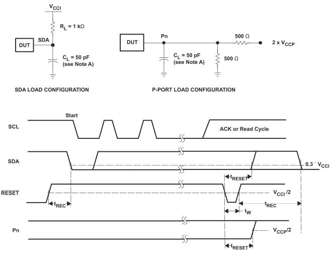
A.  $C_L$  includes probe and jig capacitance.
