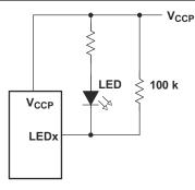
Figure 8-2. High-Value Resistor in Parallel with LED
