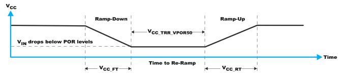
Figure 9-7. V is lowered below the POR threshold, then ramped back up
