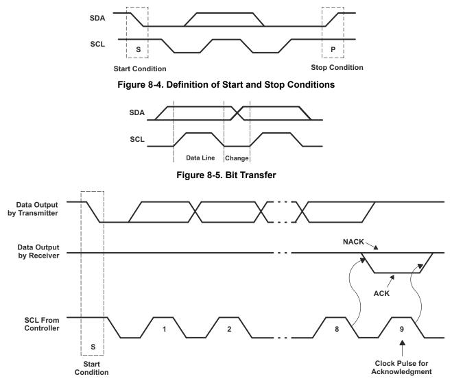
Figure 8-6. Acknowledgment on the I<sup>2</sup>C Bus
