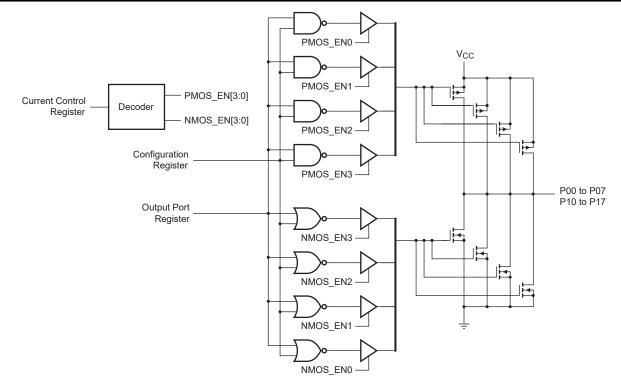
Figure 8-3. Simplified output stage
