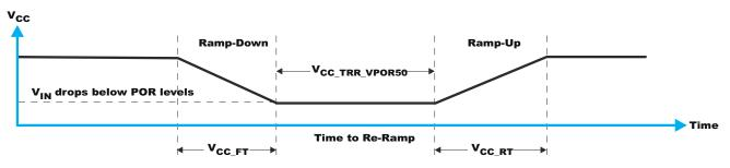
Figure 9-7. V is lowered below the POR threshold, then ramped back up
