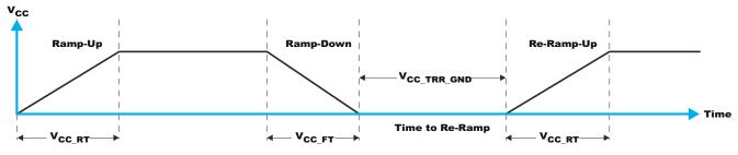
Figure 9-6. V is lowered below 0.2 V or 0 V and then ramped up
