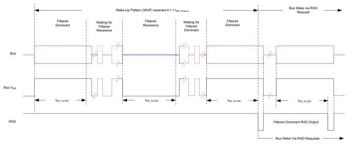
Figure 8-5. Wake-Up Pattern (WUP) with  $t_{WK_{TIMEOUT}}$
