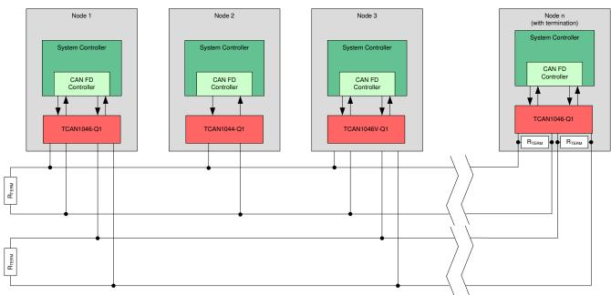
Figure 9-3. Typical CAN Bus
