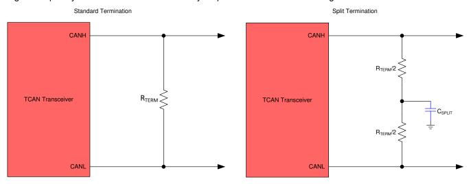
Figure 9-2. CAN Bus Termination Concepts
