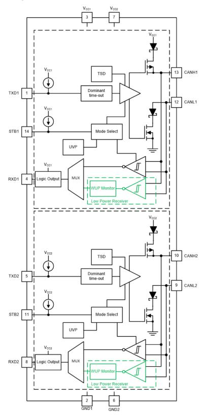
Figure 8-1. Block Diagram
