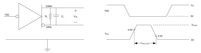
Figure 7-6. TXD Dominant Timeout Test Circuit and Measurement
