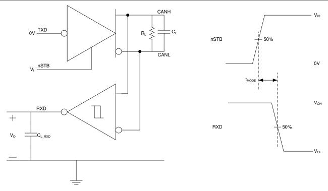
Figure 9-6. TCAN1048AV  $t_{\text{MODE}}$  Test Circuit and Measurement
