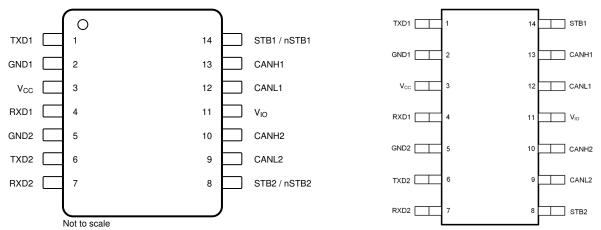
Figure 7-1. D Package, 14 Pin SOIC, Top View
