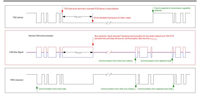
Figure 10-4. Example Timing Diagram for TXD Dominant Timeout
