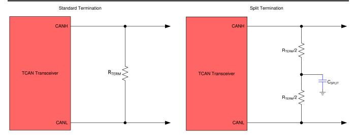
Figure 11-2. CAN Bus Termination Concepts
