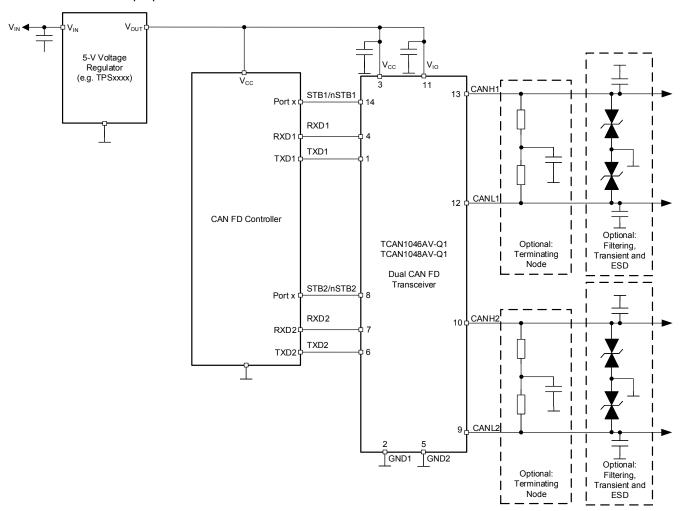
Figure 11-1. Transceiver Application Using 5 V I/O Connections
