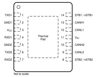
Figure 7-3. DMT Package, 14 Pin VSON, Top View
