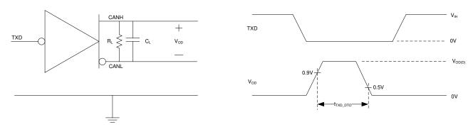
Figure 9-7. TXD Dominant Timeout Test Circuit and Measurement
