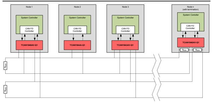
Figure 11-3. Typical CAN Bus
