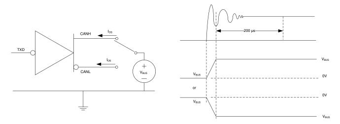
Figure 9-8. Driver Short-Circuit Current Test and Measurement
