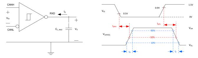
Figure 9-3. Receiver Test Circuit and Measurement
