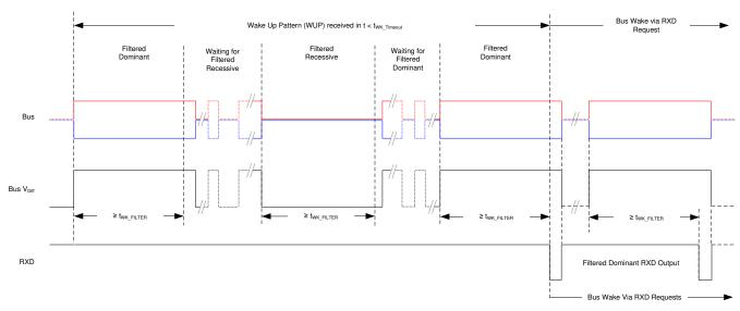
Figure 10-5. Wake-Up Pattern (WUP) with twk TIMEOUT
