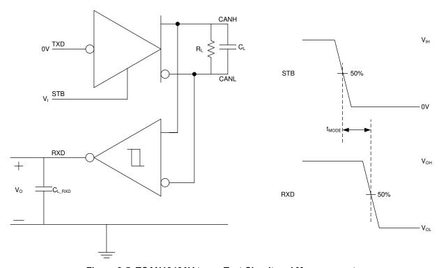
Figure 9-5. TCAN1046AV  $t_{\mbox{\scriptsize MODE}}$  Test Circuit and Measurement
