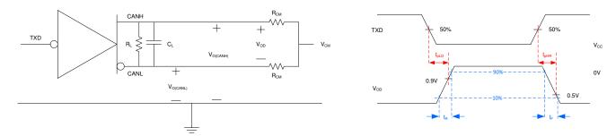
Figure 9-2. Driver Test Circuit and Measurement
