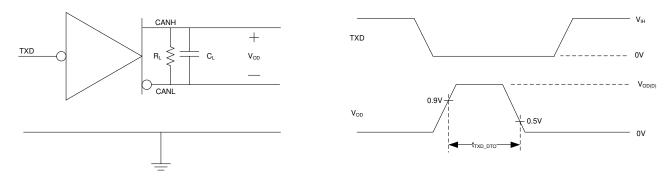
Figure 8-5. TXD Dominant Timeout Test Circuit and Measurement
