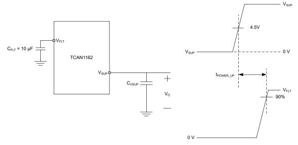
Figure 8-7. t<sub>POWER\_UP</sub> Timing Measurement
