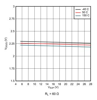
Figure 10-3. V<sub>OD(D)</sub> over V<sub>SUP</sub>
