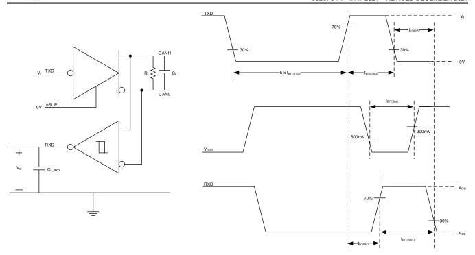
Figure 8-4. Transmitter and Receiver Timing Behavior Test Circuit and Measurement
