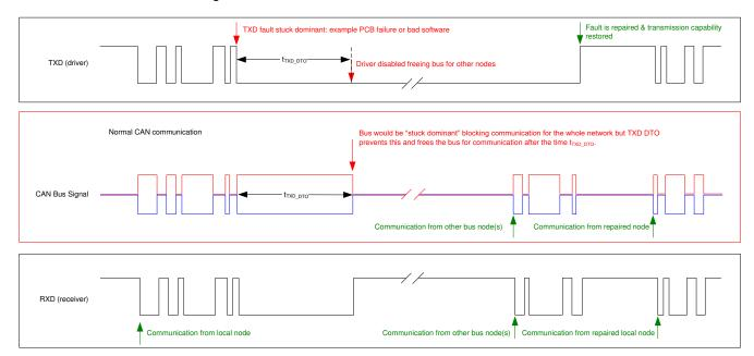
Figure 9-2. Timing Diagram for TXD DTO
