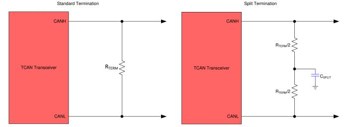
Figure 10-2. CAN Bus Termination Concepts
