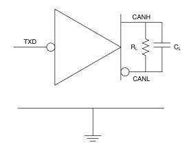
Figure 8-1. I<sub>SUP</sub> Test Circuit
