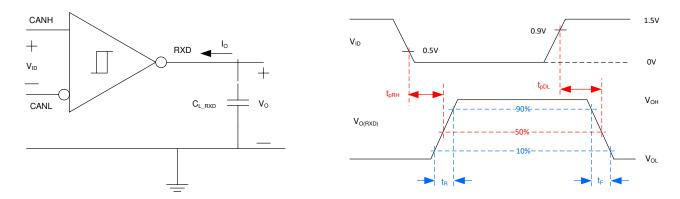
Figure 8-3. Receiver Test Circuit and Measurement
