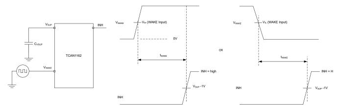
Figure 8-8. t<sub>WAKE</sub> While Monitoring INH Output
