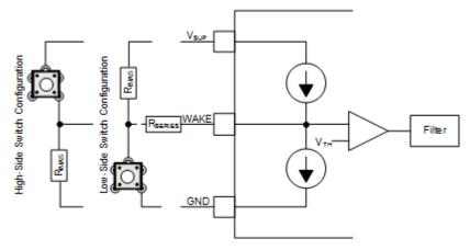
Figure 9-5. WAKE Circuit Example
