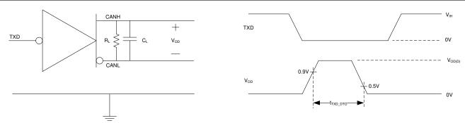
Figure 6-6. TXD Dominant Timeout Test Circuit and Measurement
