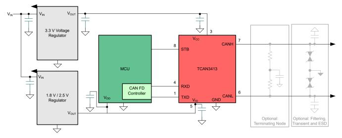
Figure 8-7. Typical Transceiver Application Using 1.8-V, 2.5-V I/O Connections
