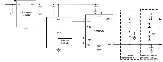
Figure 8-1. Transceiver Application Using 3.3-V I/O Connections
