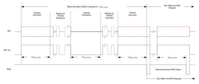
Figure 7-5. Wake-Up Pattern (WUP) with t<sub>WK\_TIMEOUT</sub>
