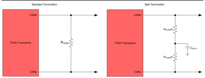
Figure 8-2. CAN Bus Termination Concepts
