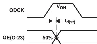
Figure 5. ODCK High to QE[23:0] Staggered Data Output
