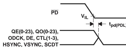
Figure 7. Delay from  $\overline{PD}$  Low to Hi-Z Outputs
