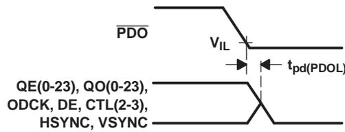
**Figure 8. Delay from  $\overline{\text{PDO}}$  Low to Hi-Z Outputs**
