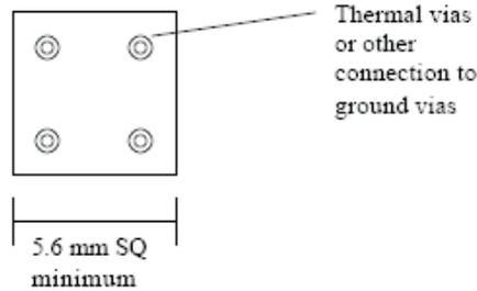
More information on this package and other requirements for using thermal lands and thermal vias are detailed in the TI application report PowerPAD™ *Thermally Enhanced Package Application Report*, TI literature number SLMA002, available via the TI Web pages beginning at [www.ti.com](http://www.ti.com).
