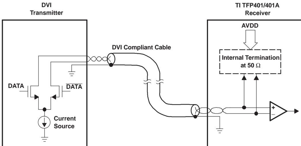
Figure 14. TMDs Differential Input and Transmitter Connection
