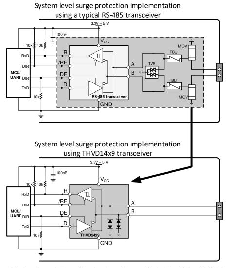
Figure 9-3. Implementation of System-Level Surge Protection Using THVD14x9(V)
