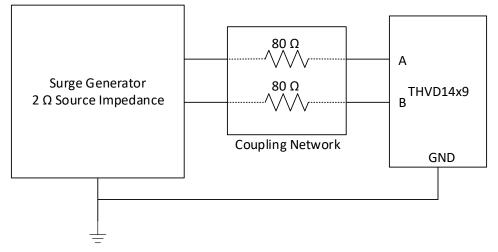
Figure 8-6. THVD14x9(V) Surge Test Setup
