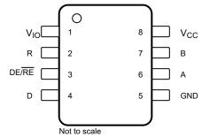
Figure 5-1. THVD1439, THVD1449, 8-Pin (SOIC), Top View
