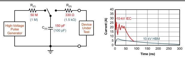
Figure 8-3. HBM and IEC ESD Models and Currents in Comparison (HBM Values in Parenthesis)
