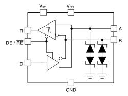
Figure 8-2. THVD1439V and THVD1449V Block Diagram
