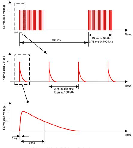
Figure 8-4. EFT Voltage Waveforms
