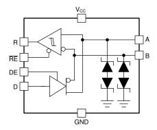
Figure 8-1. THVD1439 and THVD1449 Block Diagram
