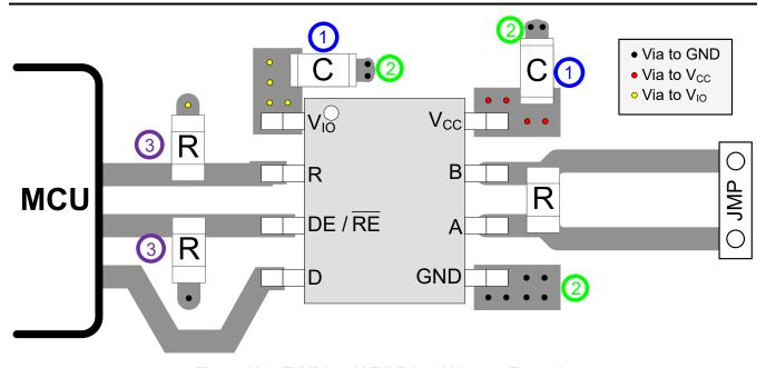
Figure 11-2. THVD1439V THVD1449V Layout Example
