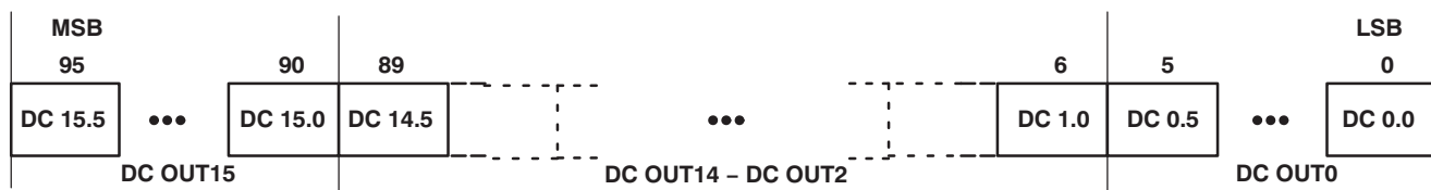
Figure 15. Dot Correction Data Packet Format
