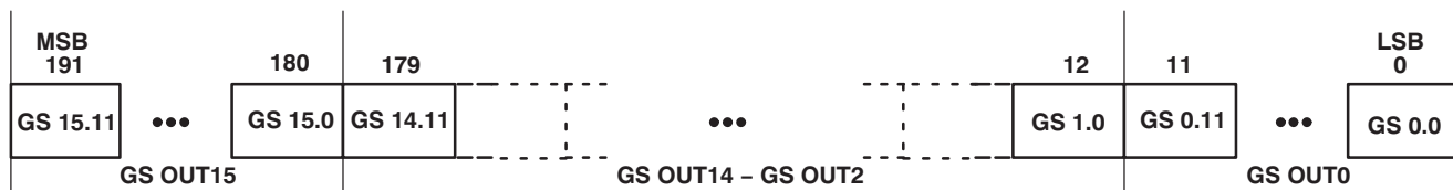
Figure 19. Grayscale Data Packet Format
