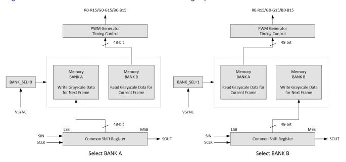
Figure 8-26. Bank Selection Exchange Operation
