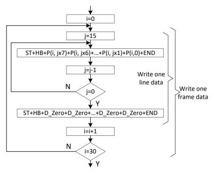
Figure 9-4. Data Write Flow
