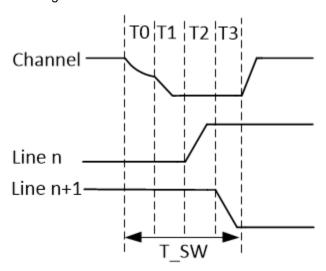
Figure 8-7. Line Transitioning Sequence
