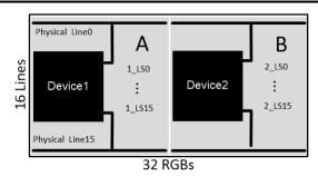
Figure 8-1. Two Devices in Independent Mode
