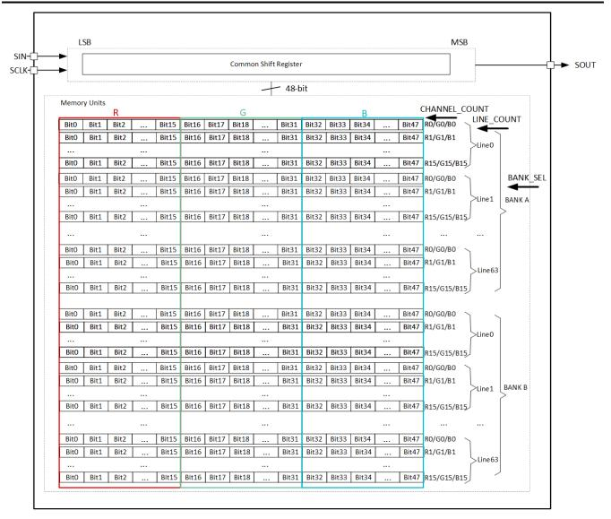
Figure 8-27. TLC6984 Memory-unit Structure
