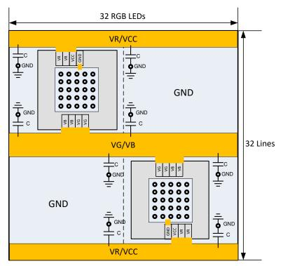
Figure 11-1. Power Rails Routing Suggestion
