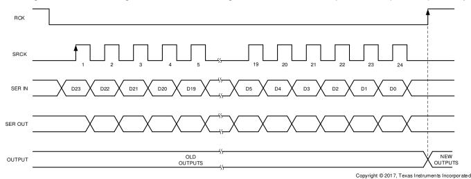
Figure 15. Register Write Timing Diagram
