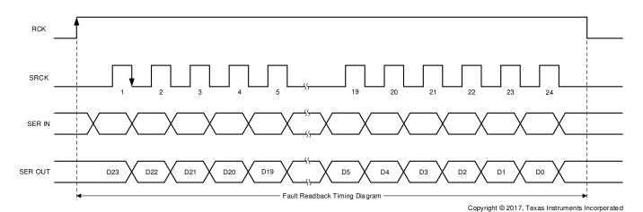
Figure 16. Register Read Timing Diagram
