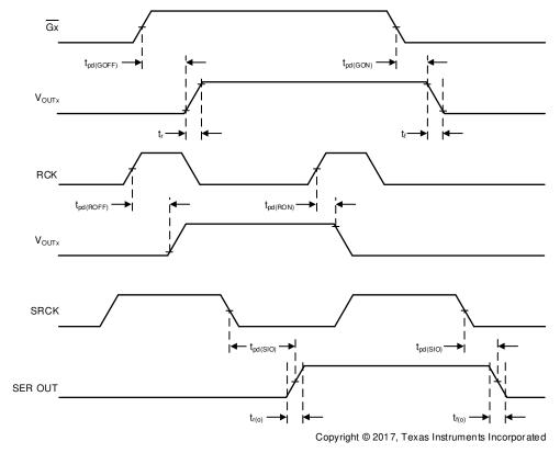
Figure 2. Timing Diagram of Output Signals
