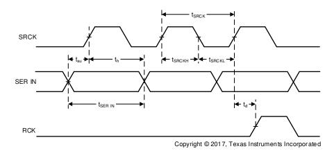
Figure 1. Timing Diagram of Input Signals
