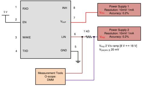
Figure 8-7. Test Circuit for  $I_{BUS\_PAS\_rec}$  Param 14
