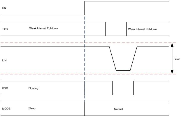
Figure 8-13. Wake-up Through EN
