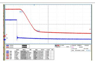
Figure 10-3. Recessive to Dominant Propagation Delay
