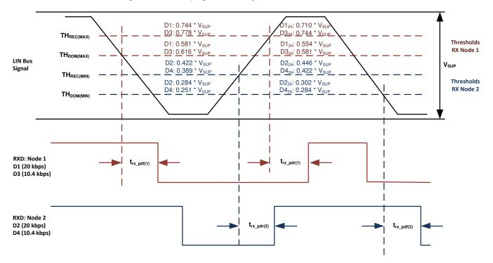
Figure 8-11. Propagation Delay
