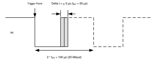
Figure 8-2. RX Response: Operating Voltage Range
