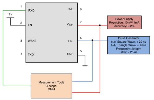
Figure 8-4. LIN Receiver Test with RX access Param 17, 18, 19, 20
