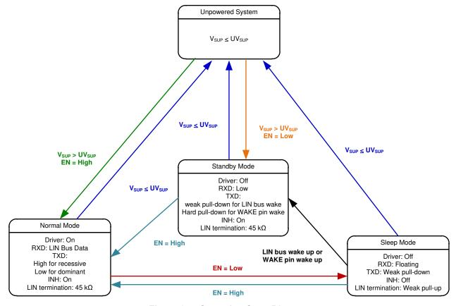
Figure 9-4. Operating State Diagram
