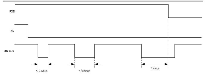
Figure 9-2. No Bus Fault: Entering Sleep Mode with Bus Recessive Condition and Wake-up
