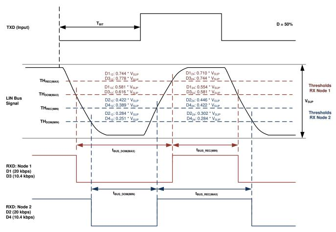
Figure 8-9. Definition of Bus Timing Parameters
