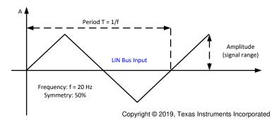
Figure 8-3. LIN Bus Input Signal
