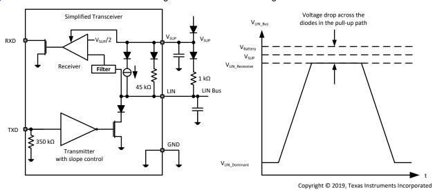
Figure 9-1. Commander Node Configuration with Voltage Levels
