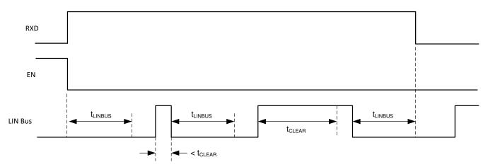
Figure 9-3. Bus Fault: Entering Sleep Mode With Bus Stuck Dominant Fault, Clearing, and Wake-up
