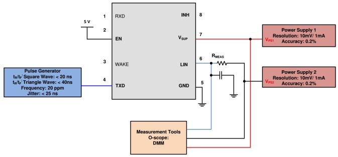
Figure 8-10. Propagation Delay Test Circuit; Param 31, 32
