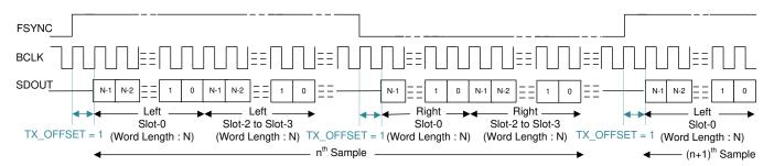
Figure 34. LJ Protocol Timing (TX\_OFFSET = 1 and BCLK\_POL = 1)
