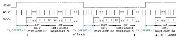
Figure 32. LJ Protocol Timing (TX\_OFFSET = 2)
