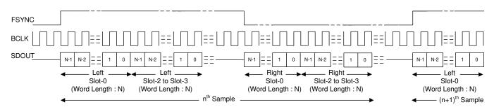
Figure 31. LJ Mode Standard Protocol Timing (TX\_OFFSET = 0)
