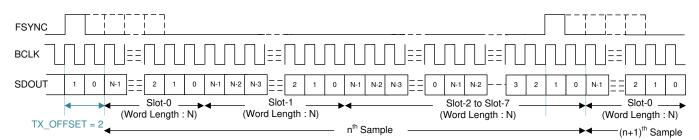
Figure 25. TDM Mode Protocol Timing (No Idle BCLK Cycles, TX OFFSET = 2)
