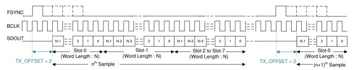
Figure 24. TDM Mode Protocol Timing (TX\_OFFSET = 2)
