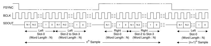
Figure 27. I<sup>2</sup>S Mode Standard Protocol Timing (TX\_OFFSET = 0)
