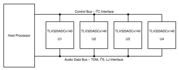
Figure 35. Multiple TLV320ADC6140 Devices With Shared Control and Audio Data Buses
