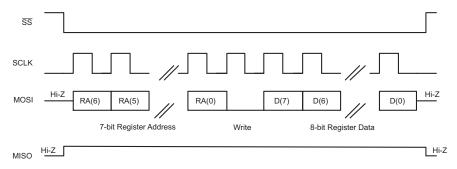
Figure 93. SPI Single-Byte Write Transfer
