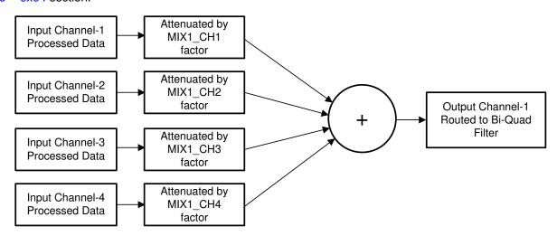
Figure 40. Programmable Digital Mixer Block Diagram
