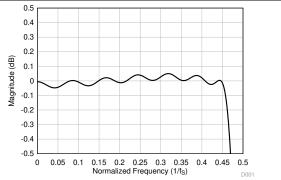
Figure 43. Linear Phase Decimation Filter Magnitude Response
