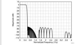
Figure 41. Linear Phase Decimation Filter Magnitude Response
