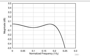
Figure 56. Linear Phase Decimation Filter Pass-Band Ripple
