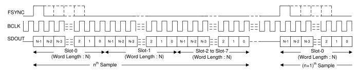
Figure 26. TDM Mode Protocol Timing (TX\_OFFSET = 0 and BCLK\_POL = 1)
