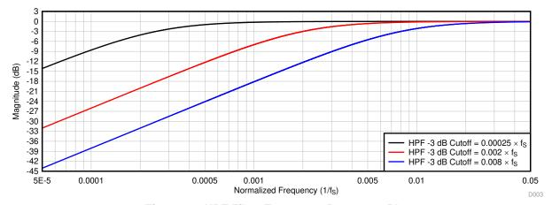
Figure 39. HPF Filter Frequency Response Plot
