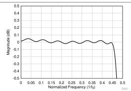
Figure 42. Linear Phase Decimation Filter Pass-Band Ripple
