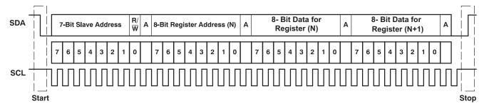
Figure 88. Typical I<sup>2</sup>C Sequence
