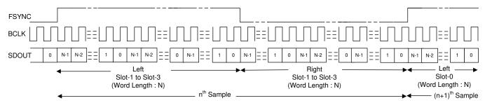
Figure 33. LJ Protocol Timing (No Idle BCLK Cycles, TX OFFSET = 0)
