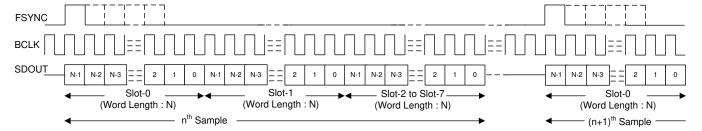
Figure 23. TDM Mode Standard Protocol Timing (TX OFFSET = 0)
