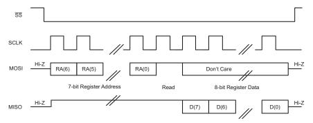
Figure 94. SPI Single-Byte Read Transfer
