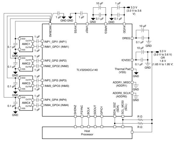
Figure 172. Four-Channel Analog Microphone Recording Diagram
