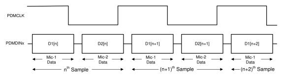
Figure 87. Digital PDM Microphone Protocol Timing Diagram
