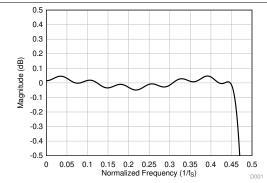
Figure 49. Linear Phase Decimation Filter Magnitude Response
