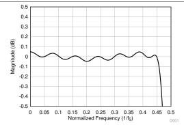
Figure 45. Linear Phase Decimation Filter Magnitude Response
