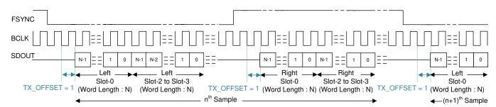
Figure 28. I<sup>2</sup>S Protocol Timing (TX\_OFFSET = 1)
