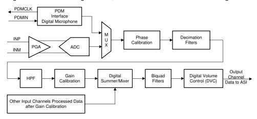
Figure 38. Signal-Chain Processing Flowchart
