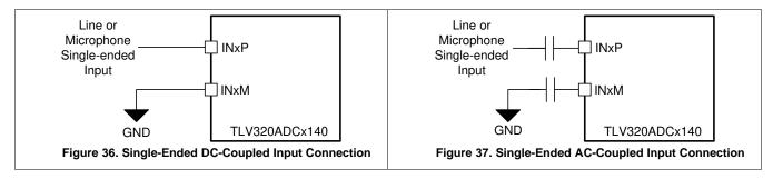
The device allows for flexibility in choosing the typical input impedance on INxP or INxM from 2.5 k $\Omega$  (default), 10 k $\Omega$ , and 20 k $\Omega$  based on the input source impedance. The higher input impedance results in slightly higher noise or lower dynamic range. Table 9 lists the configuration register settings for the input impedance for the record channel.
