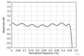
Figure 51. Linear Phase Decimation Filter Magnitude Response
