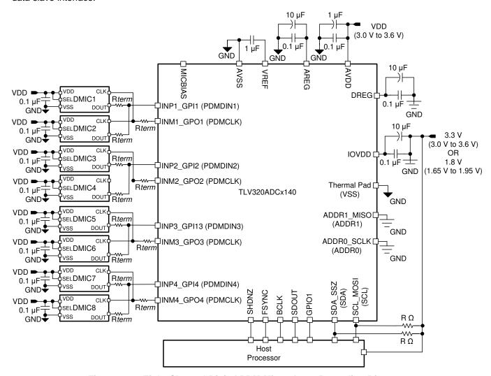
Figure 177. Eight-Channel Digital PDM Microphone Recording Diagram
