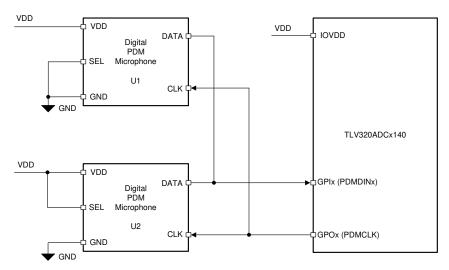
Figure 86. Digital PDM Microphones Connection Diagram to the TLV320ADC6140
