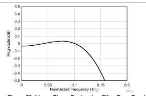
Figure 58. Linear Phase Decimation Filter Pass-Band
