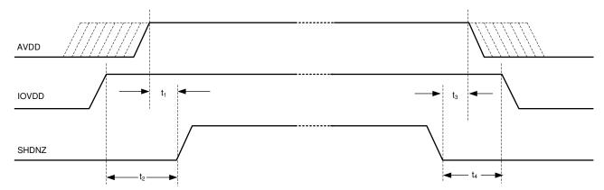
Figure 178. Power-Supply Sequencing Requirement Timing Diagram
