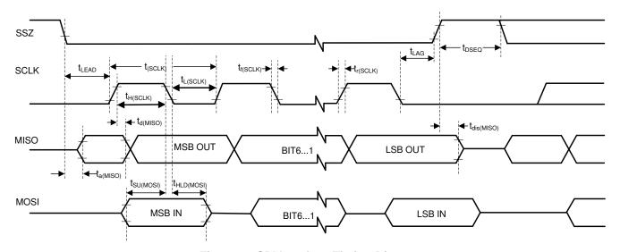
Figure 2. SPI Interface Timing Diagram
