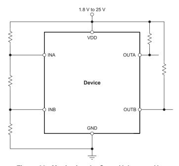
Figure 22. Monitoring the Same Voltage as  $V_{\text{DD}}$
