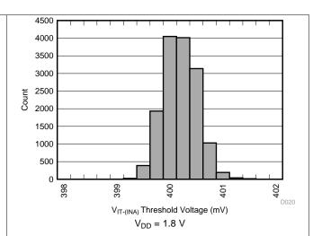
Figure 9. INA Negative Input Threshold Voltage (V<sub>IT-(INA)</sub>)
