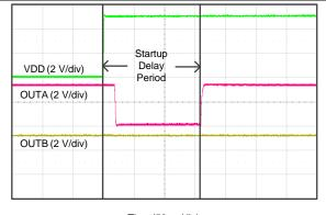
Time (50 µs/div)  $V_{DD}$  = 5 V,  $V_{INA}$  = 410 mV,  $V_{INB}$  = 390 mV,  $V_{PULLUP}$  = 3.3 V
