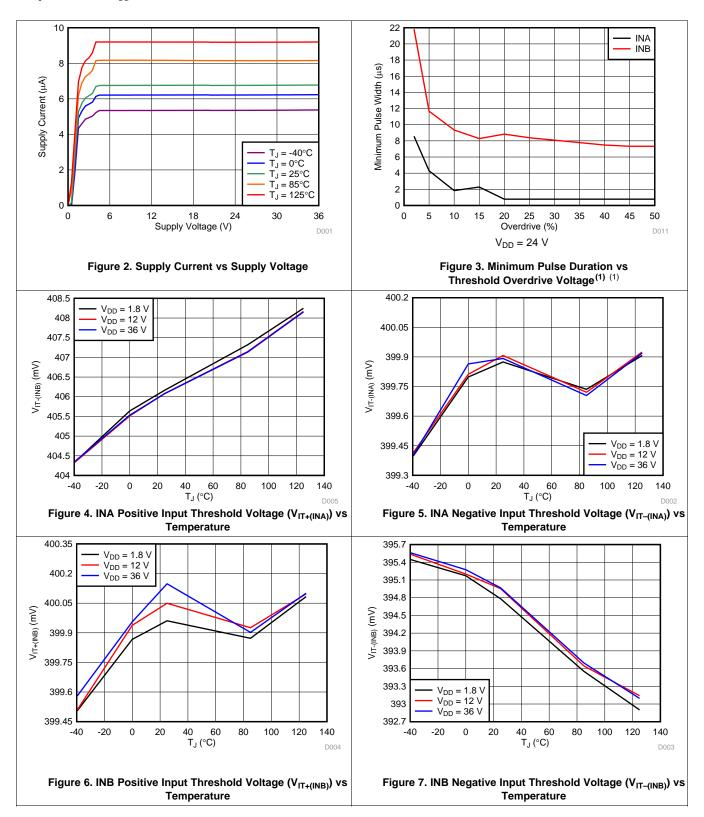
(1) Minimum pulse duration required to trigger output high-to-low transition. INA = negative spike below  $V_{IT-}$  and INB = positive spike above  $V_{IT+}$ .
