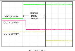
Time (50 µs/div)  $V_{DD}$  = 5 V,  $V_{INA}$  = 390 mV,  $V_{INB}$  = 410 mV,  $V_{PULLUP}$  = 3.3 V
