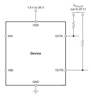
Figure 21. Interfacing to Voltages Other than  $V_{\text{DD}}$
