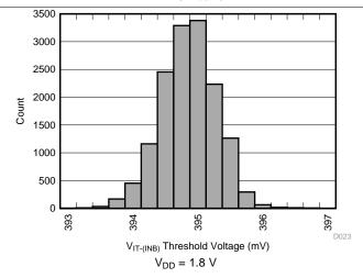
Figure 11. INB Negative Input Threshold Voltage (V<sub>IT-(INB)</sub>)
