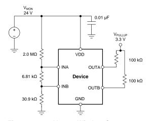
Figure 24. 24-V, 10% Window Comparator
