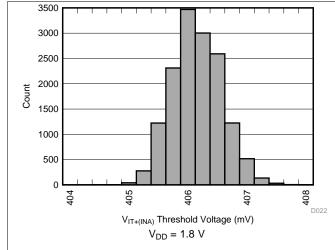
Figure 8. INA Positive Input Threshold Voltage (V<sub>IT+(INA)</sub>)
