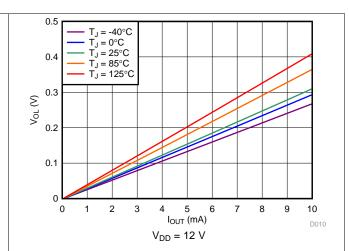
Figure 14. Output Voltage Low vs Output Sink Current
