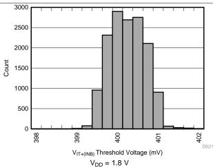
Figure 10. INB Positive Input Threshold Voltage (V<sub>IT+(INB)</sub>)
