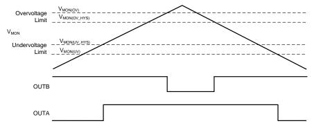
Figure 20. Window Comparator Timing Diagram
