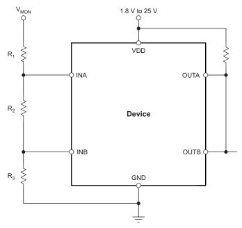
NOTE: The inputs can monitor a voltage higher than  $V_{DD}$  (max) with the use of an external resistor divider network.
