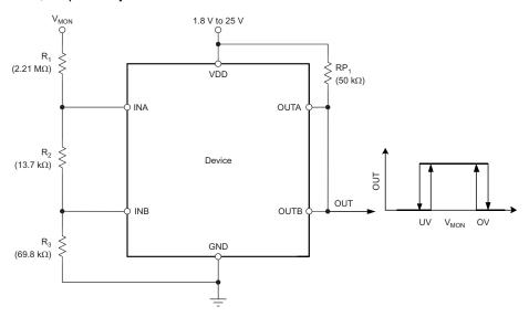
Figure 19. Window Comparator Block Diagram
