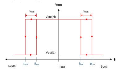
Figure 8-3. Omnipolar Functionality
