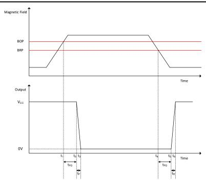
Figure 8-8. Propagation Delay
