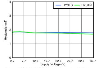
Figure 7-14. TMAG5123D Hysteresis vs. Supply Voltage
