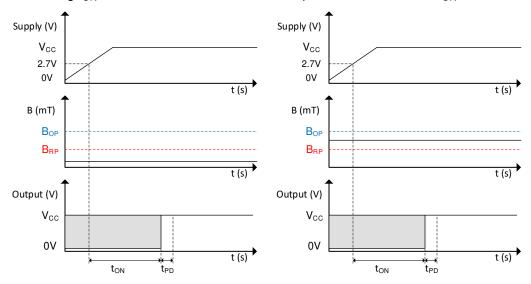
Figure 8-5. Power-On Time When  $B < B_{OP}$
