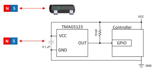
Figure 9-1. Typical In-Plane Sensing Diagram
