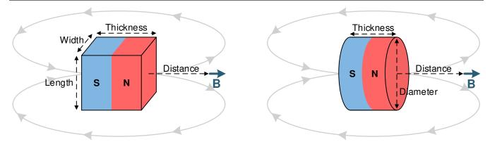
Figure 9-2. Rectangular Block and Cylinder Magnets
