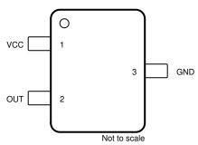
Figure 6-1. DBZ Package 3-Pin SOT-23 Top View
