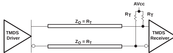
Figure 1. Termination for TMD5 Output Driver
