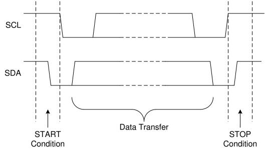
Figure 7-7. Definition of Start and Stop Conditions
