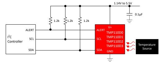
Figure 9-2. Equal I<sup>2</sup>C Pullup and Supply Voltage Application
