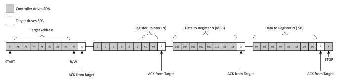
Figure 7-9. Write to Single Register
