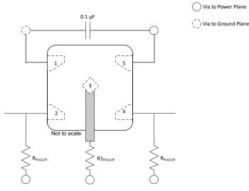
Figure 9-4. ALERT Pin Layout Example
