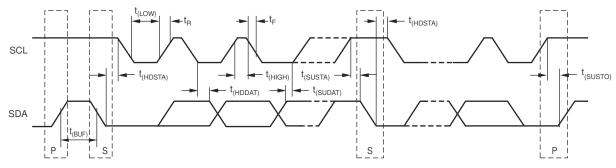
Figure 6-1. Two-Wire Timing Diagram
