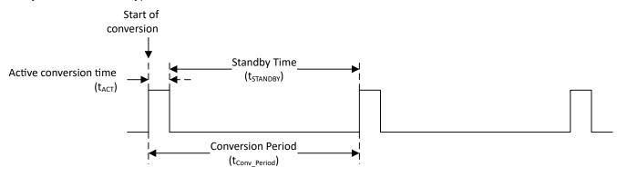
Figure 7-5. Continuous Conversion Cycle Timing Diagram
