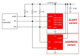
Figure 3-1. Simplified Schematic
