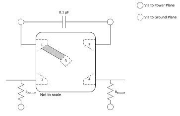
Figure 9-3. ADD0 Pin Layout Example
