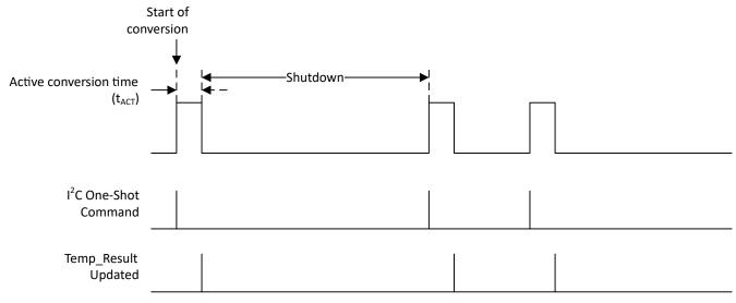
Figure 7-6. One-Shot Timing Diagram
