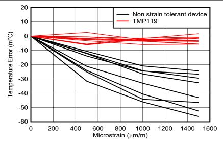
Figure 7-3. Strain Tolerance
