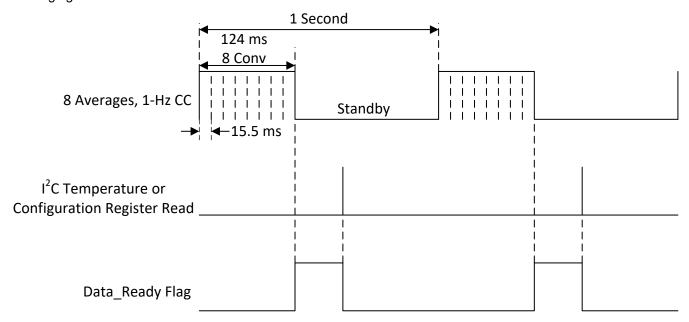
Figure 7-2. Averaging Timing Diagram
