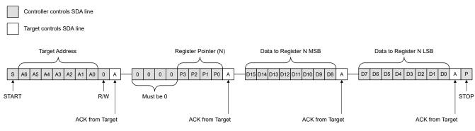
Figure 7-10. Write Word Command Timing Diagram
