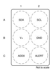
Figure 5-1. YBG Package 6-Pin DSBGA Top View
