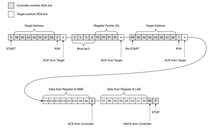
Figure 7-11. Read Word Command Timing Diagram
