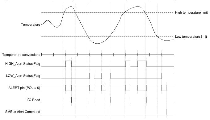
Figure 7-6. Alert Mode Timing Diagram
