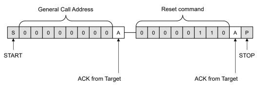
Figure 7-13. General-Call Reset Command Timing Diagram
