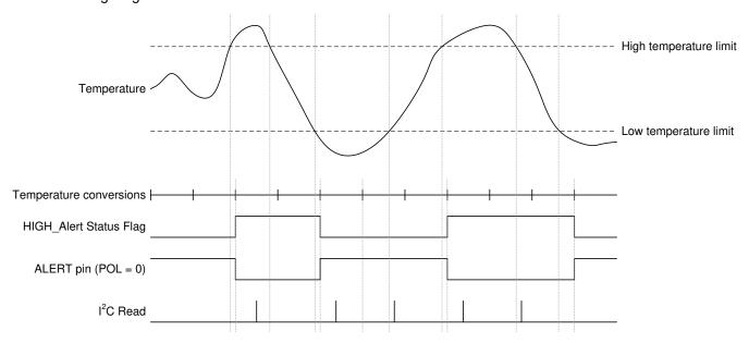
Figure 7-7. Therm Mode Timing Diagram
