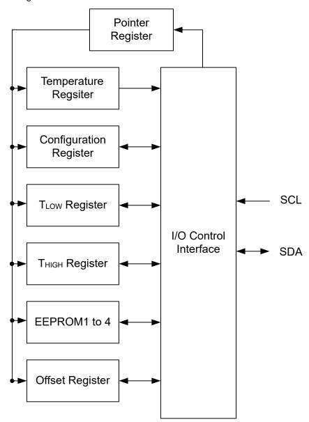
Figure 7-9. Internal Register Structures
