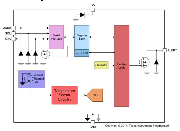
Figure 7-1. Internal Block Diagram
