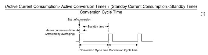
Figure 7-4. Conversion Cycle Timing Diagram
