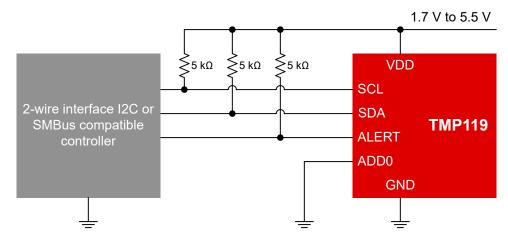
Figure 8-2. Typical Connections
