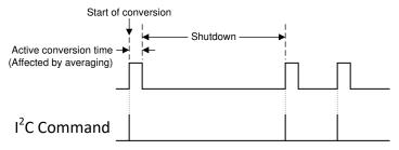
Figure 7-5. One-Shot Timing Diagram With AVG[1:0] = 00
