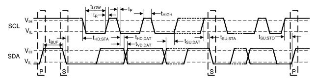
Figure 6-1. Two-Wire Timing Diagram
