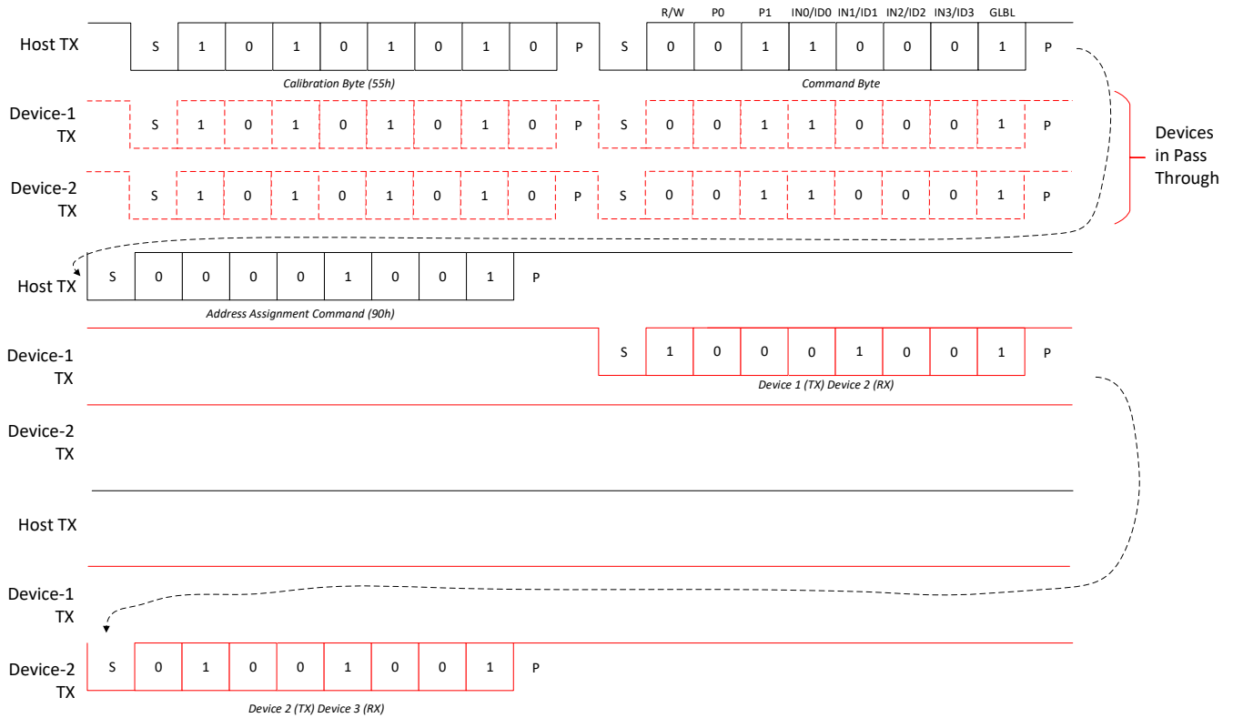
Figure 7-8. Global Initialization and Address Assignment Command Flow
