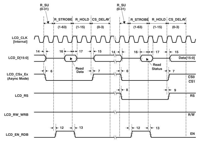
Figure 5-29. Micro-Interface Graphic Display 6800 Status
