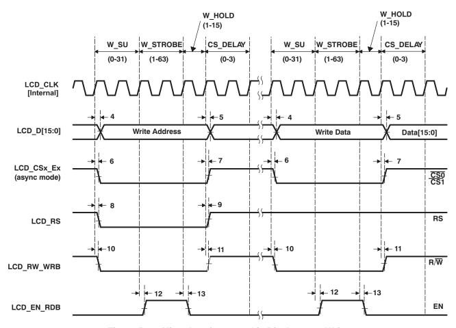
Figure 5-27. Micro-Interface Graphic Display 6800 Write
