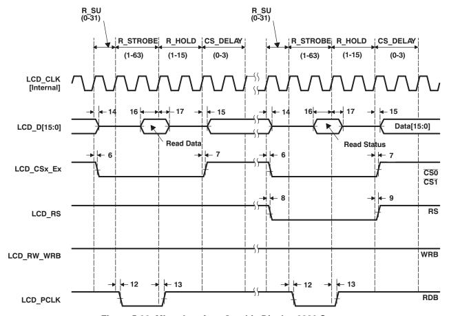
Figure 5-32. Micro-Interface Graphic Display 8080 Status
