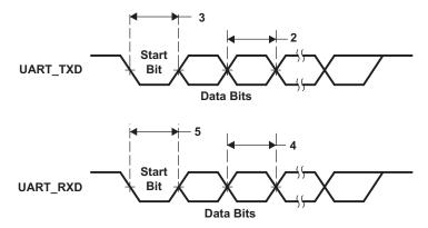
Figure 5-41. UART Transmit and Receive Timing
