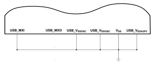
Figure 5-15. Connections when USB Oscillator is Permanently Disabled
