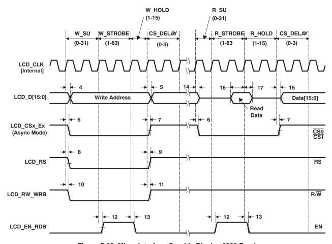
Figure 5-28. Micro-Interface Graphic Display 6800 Read
