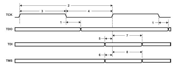
Figure 5-43. JTAG Test-Port Timing
