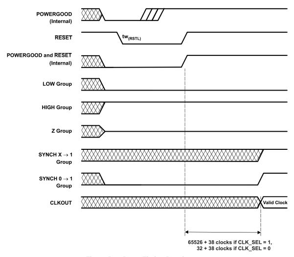
Figure 5-9. Reset Timing Requirements
