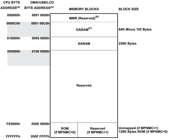
A. The USB and LCD controllers do not have access to DARAM.
