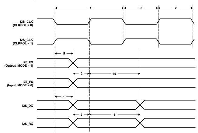
Figure 5-24. I2S Input and Output Timings
