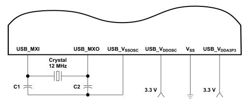
Figure 5-14. 12-MHz USB Oscillator
