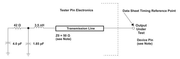
NOTE: The data sheet provides timing at the device pin. For output timing analysis, the tester pin electronics and its transmission line effects must be taken into account. A transmission line with a delay of 2 ns can be used to produce the desired transmission line effect. The transmission line is intended as a load only. It is not necessary to add or subtract the transmission line delay (2 ns) from the data sheet timings.
