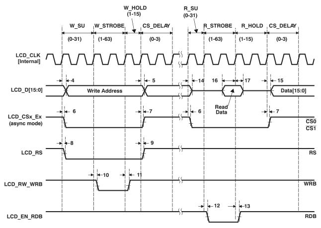
Figure 5-31. Micro-Interface Graphic Display 8080 Read
