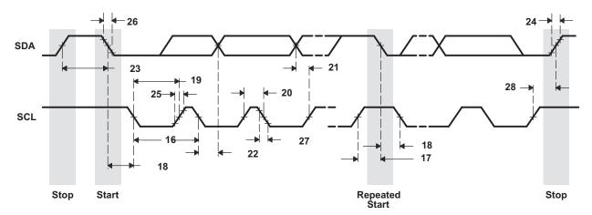
Figure 5-23. I2C Transmit Timings
