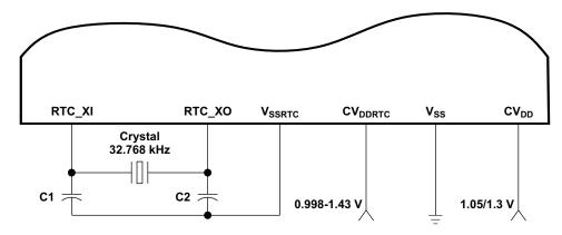
Figure 5-11. 32.768-kHz RTC Oscillator
