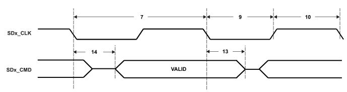
Figure 5-33. SD Host Command Write Timing
