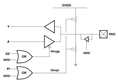
Figure 5-7. Bus Holder I/O Circuit
