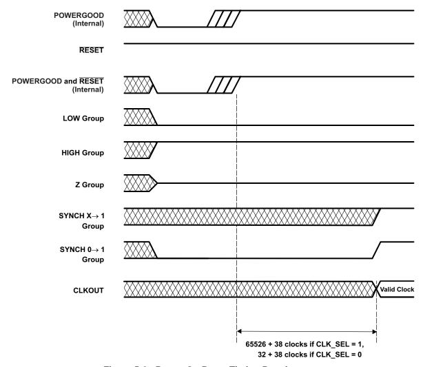
Figure 5-8. Power-On Reset Timing Requirements
