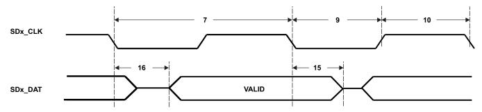
Figure 5-36. SD Data Write Timing
