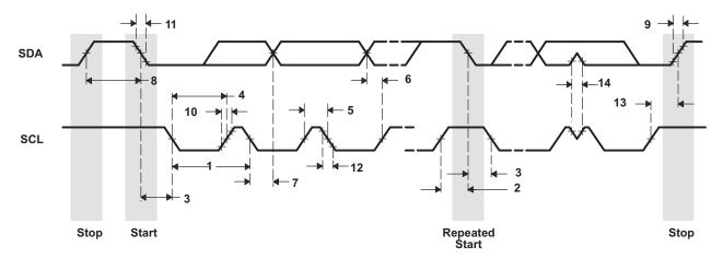
Figure 5-22. I2C Receive Timings
