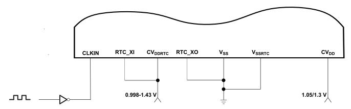
Figure 5-13. LVCMOS-Compatible Clock Input With RTC Oscillator Disabled
