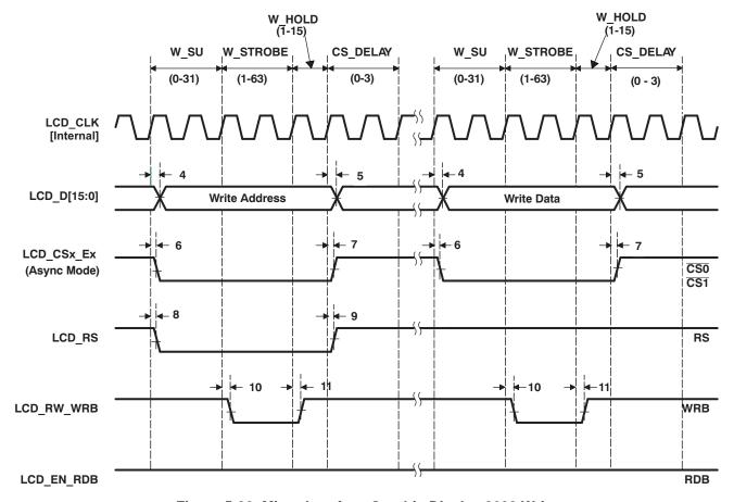
Figure 5-30. Micro-Interface Graphic Display 8080 Write
