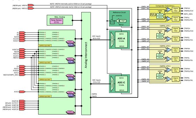
Figure 6-37. Analog Subsystem Block Diagram
