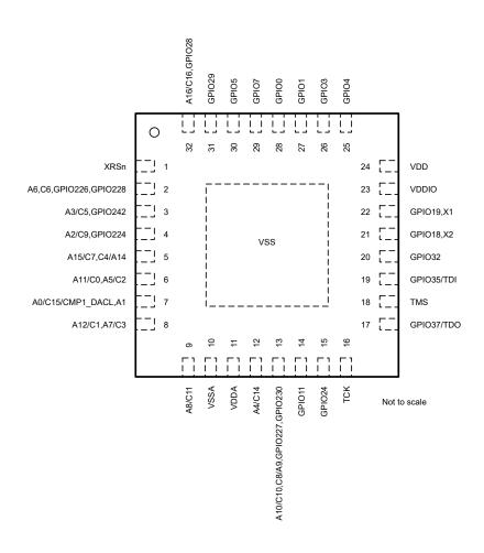
Figure 5-5. 32-Pin RHB Very Thin Quad Flatpack No Lead (Top View)
