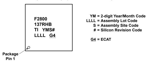
Figure 9-5. Package Symbolization for RHB Package
