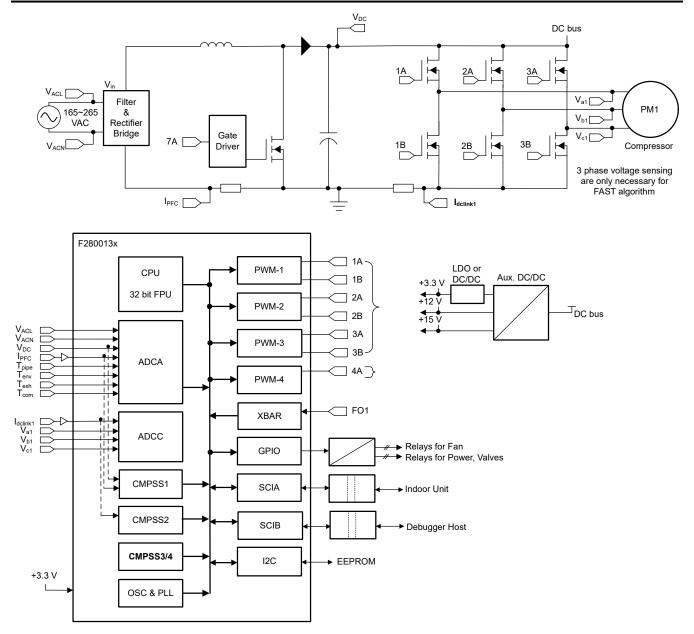
Figure 8-3. Typical Variable-Frequency Air-Conditioner with Single-Motor Control Using Single Shunt
