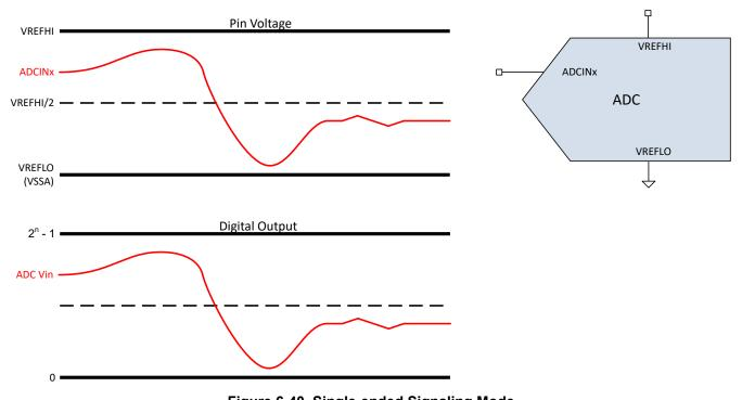
Figure 6-40. Single-ended Signaling Mode
