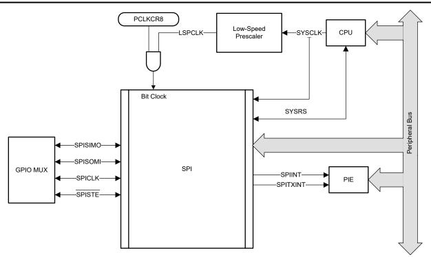
Figure 6-69. SPI CPU Interface
