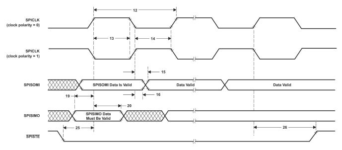
Figure 6-73. SPI Slave Mode External Timing (Clock Phase = 1)
