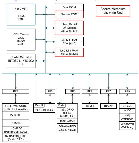
Figure 7-1. Functional Block Diagram
