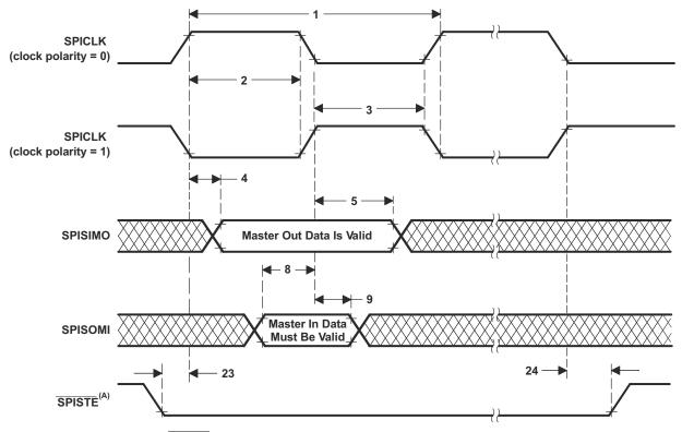
A. On the trailing end of the word, SPISTE will go inactive except between back-to-back transmit words in both FIFO and non-FIFO modes.
