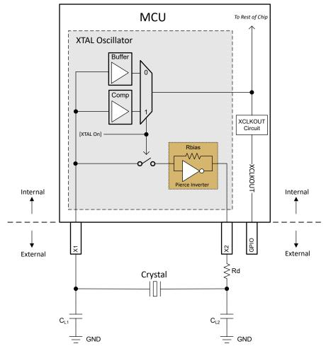
Figure 6-17. Electrical Oscillator Block Diagram
