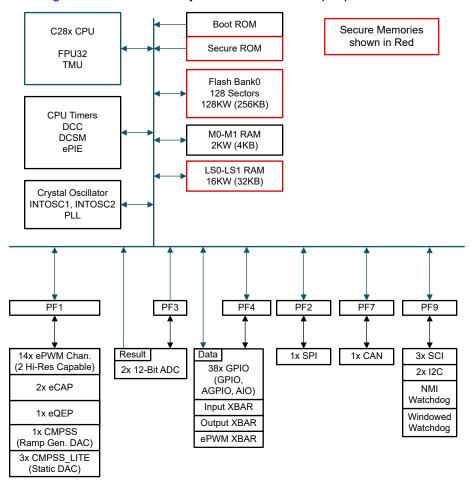
Figure 3-1. Functional Block Diagram
