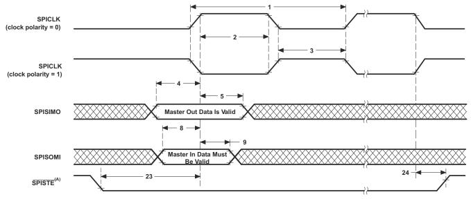
A. On the trailing end of the word, SPISTE will go inactive except between back-to-back transmit words in both FIFO and non-FIFO modes.
