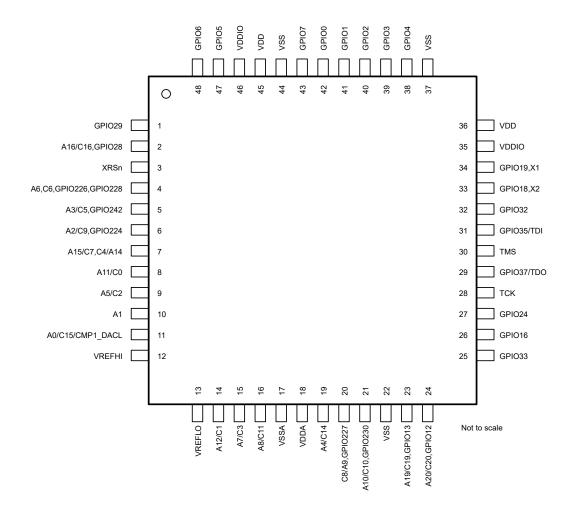
Figure 5-3. 48-Pin PT Low-Profile Quad Flatpack (Top View)
