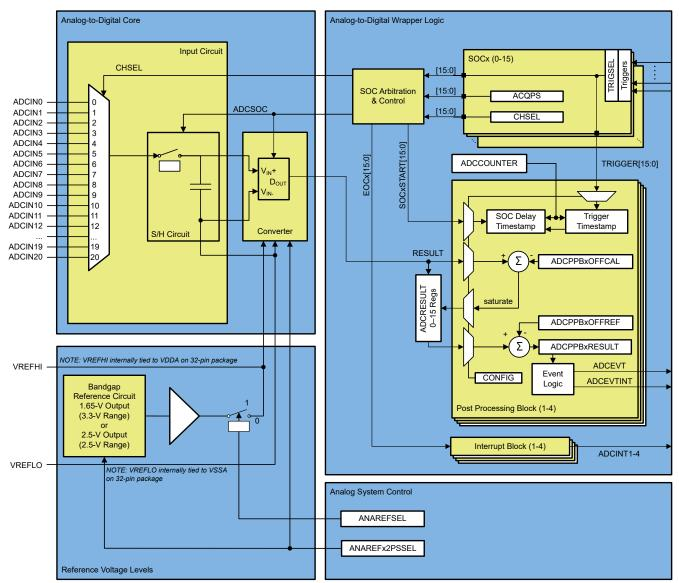
Figure 6-39. ADC Module Block Diagram
