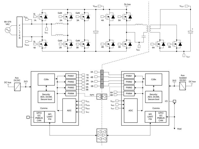
Figure 8-10. Merchant Telecom Rectifier Dual-chip Architecture
