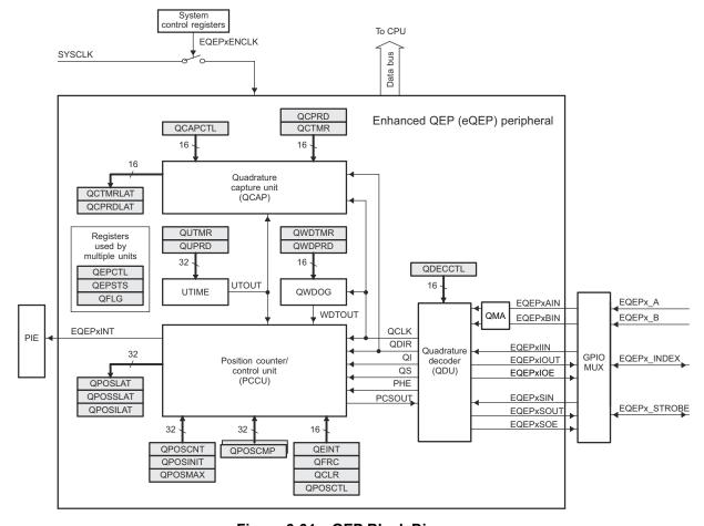
Figure 6-64. eQEP Block Diagram
