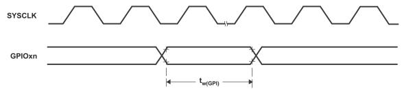
Figure 6-31. General-Purpose Input Timing
