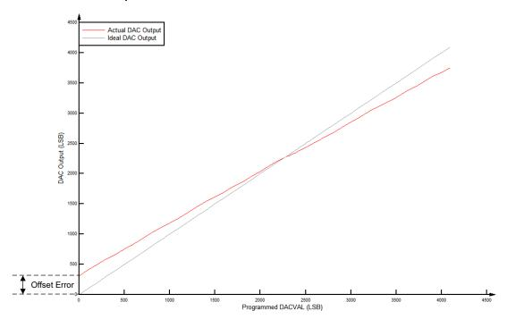
Figure 6-53. CMPSS DAC Static Offset
