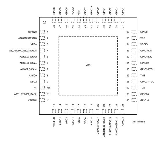
Figure 5-4. 48-Pin RGZ Very Thin Quad Flatpack No Lead (Top View)
