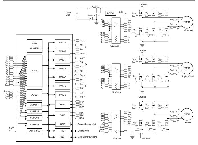
Figure 8-8. Single-Chip Solution for Robotic Lawn Mower
