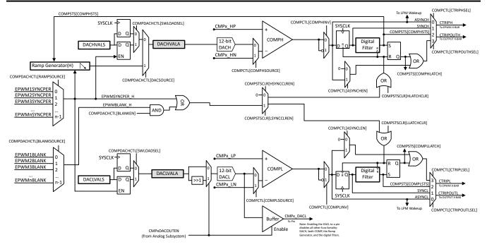
Figure 6-48. CMPSS Module Block Diagram
