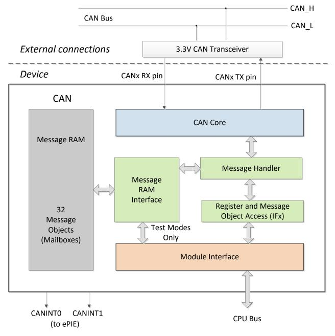
Figure 6-65. CAN Block Diagram
