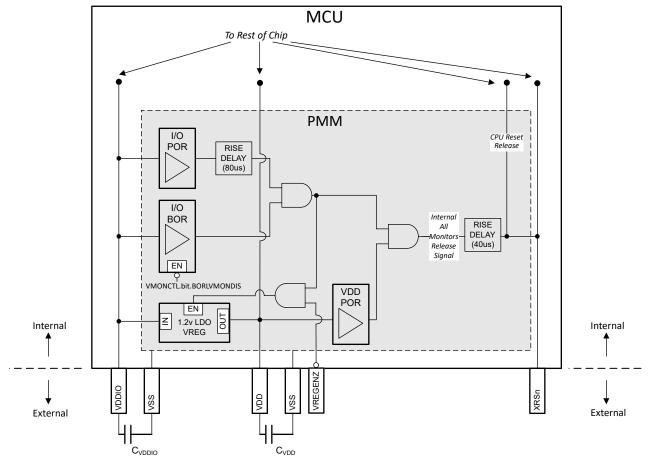
Figure 6-4. PMM Block Diagram
