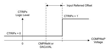
Figure 6-51. CMPSS Comparator Input Referred Offset
