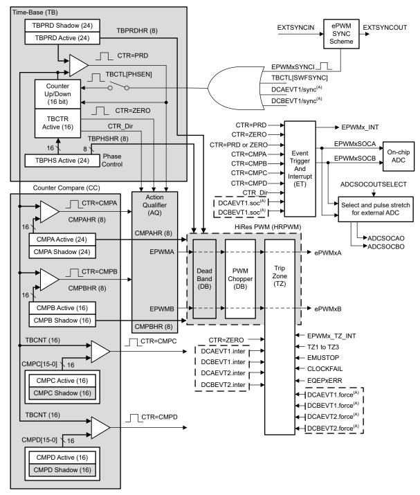
A. These events are generated by the ePWM digital compare (DC) submodule based on the levels of the TRIPIN inputs.
