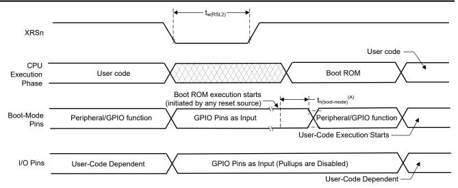
A. After reset from any source (see the Reset Sources section), the Boot ROM code samples BOOT Mode pins. Based on the status of the Boot Mode pin, the boot code branches to destination memory or boot code function. If Boot ROM code executes after power-on conditions (in debugger environment), the Boot code execution time is based on the current SYSCLK speed. The SYSCLK will be based on user environment and could be with or without PLL enabled.
