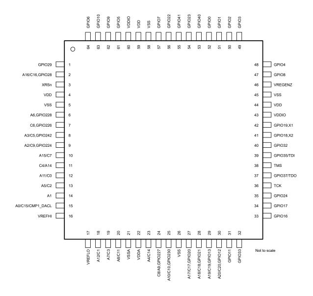
Figure 5-2. 64-Pin PM Low-Profile Quad Flatpack with VREGENZ (Top View)
