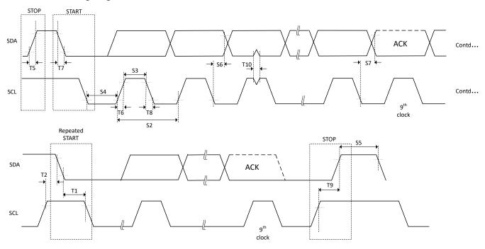
Figure 6-67. I2C Timing Diagram
