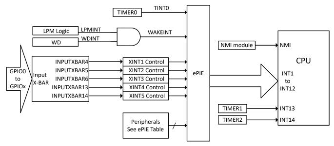
Figure 6-32. Device Interrupt Architecture
