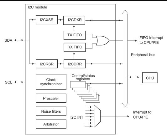
Figure 6-66. I2C Peripheral Module Interfaces
