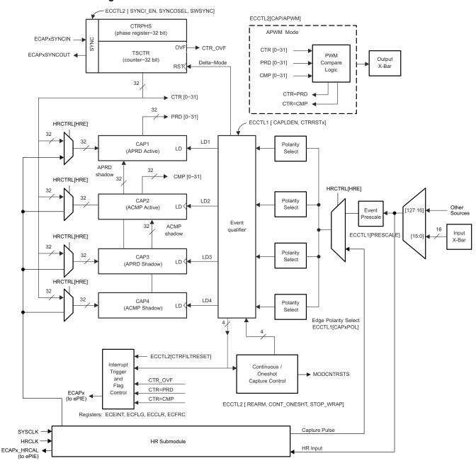
Figure 6-62. eCAP Block Diagram
