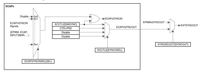
Figure 6-63. eCAP Synchronization Scheme
