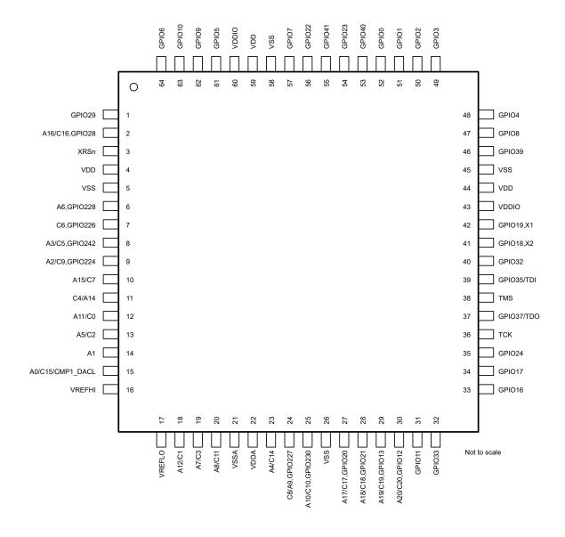
Figure 5-1. 64-Pin PM Low-Profile Quad Flatpack (Top View)
