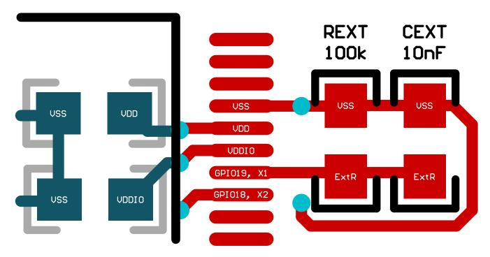
Figure 6-22. ExtR PCB Layout Example
