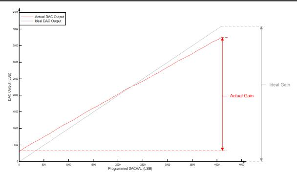
Figure 6-54. CMPSS DAC Static Gain
