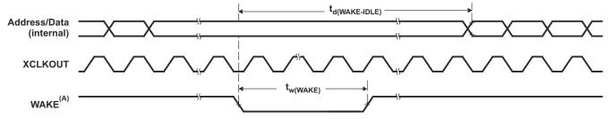
A. WAKE can be any enabled interrupt, WDINT or XRSn. After the IDLE instruction is executed, a delay of five OSCCLK cycles (minimum) is needed before the wake-up signal could be asserted.
