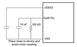
Figure 6-21. ExtR Example Schematic
