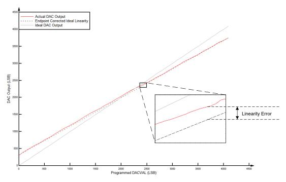
Figure 6-55. CMPSS DAC Static Linearity
