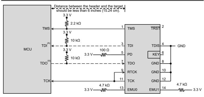
A. TDI and TDO connections are not required for cJTAG option and these pins can be used as GPIOs instead.
