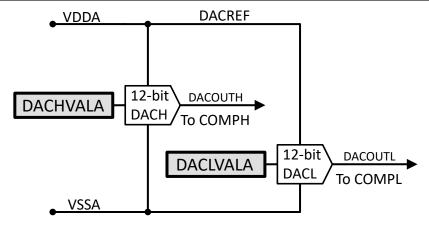
Figure 6-50. Reference DAC Block Diagram
