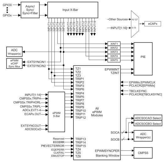
Figure 6-58. ePWM Trip Input Connectivity
