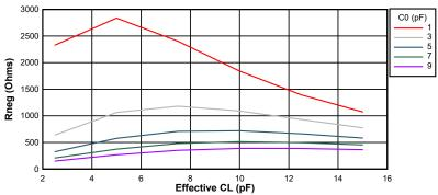
Figure 6-19. Negative Resistance Variation at 10 MHz
