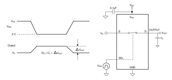
Figure 7-5. Charge-Injection Measurement Setup
