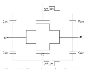
Figure 8-2. Transmission Gate Topology
