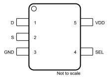
Figure 5-1. DCK Package 5-Pin SC70 (Top View)
