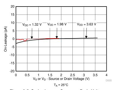
Figure 9-5. On-Leakage vs Source or Drain Voltage
