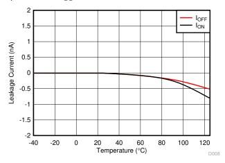
Figure 8-1. Leakage Current vs Temperature
