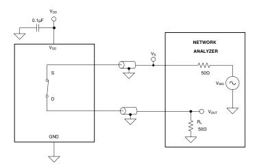
Figure 7-7. Bandwidth Measurement Setup
