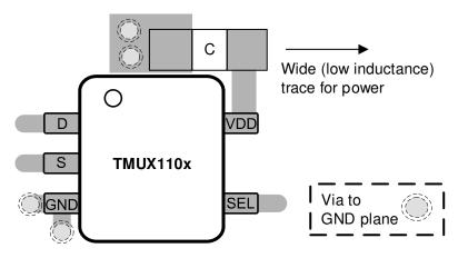
Figure 9-7. TMUX110x Layout Example
