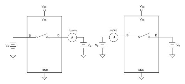
Figure 7-2. Off-Leakage Measurement Setup
