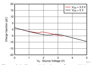
Figure 8-3. Charge Injection vs Source Voltage
