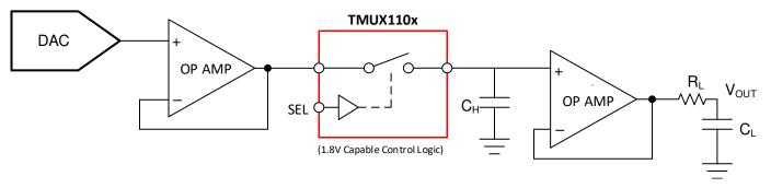
Figure 9-1. Single Channel Sample-and-Hold Circuit Example
