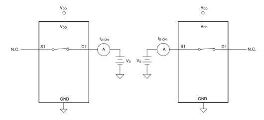
Figure 7-3. On-Leakage Measurement Setup
