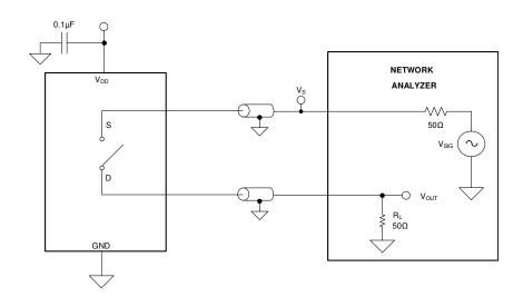
Figure 7-6. Off Isolation Measurement Setup
