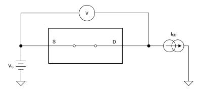
Figure 7-1. On-Resistance Measurement Setup
