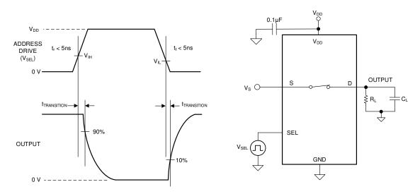
Figure 7-4. Transition-Time Measurement Setup
