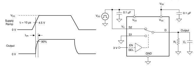
Figure 7-7. t<sub>ON (VDD)</sub> Time Measurement Setup
