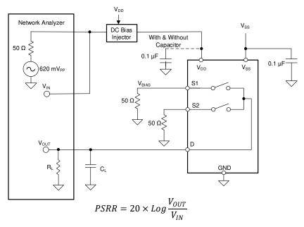
Figure 7-14. ACPSRR Measurement Setup
