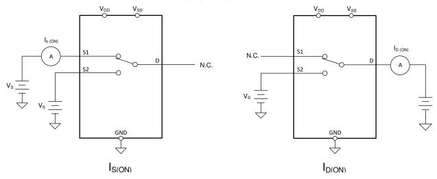
Figure 7-3. On-Leakage Measurement Setup
