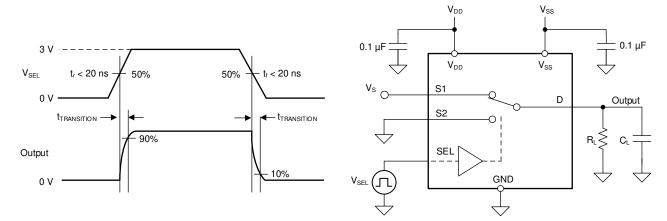
Figure 7-4. Transition-Time Measurement Setup
