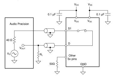
Figure 7-13. THD + N Measurement Setup
