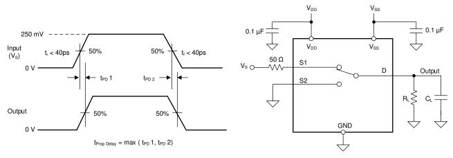
Figure 7-8. Propagation Delay Measurement Setup
