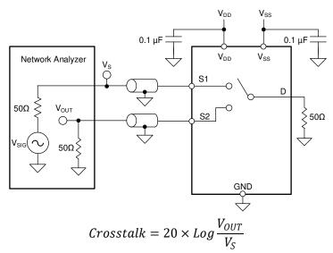
Figure 7-11. Crosstalk Measurement Setup
