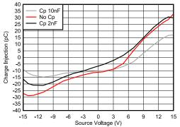
Figure 8-3. Charge Injection Compensation
