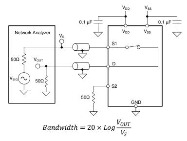
Figure 7-12. Bandwidth Measurement Setup
