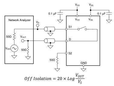
Figure 7-10. Off Isolation Measurement Setup
