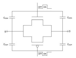
Figure 8-2. Transmission Gate Topology
