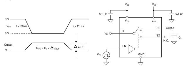
Figure 7-9. Charge-Injection Measurement Setup
