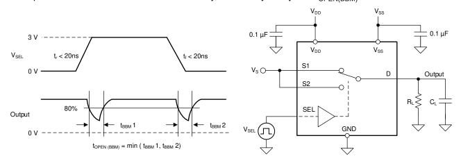
Figure 7-6. Break-Before-Make Delay Measurement Setup
