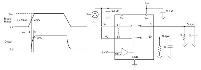
Figure 8-5. t<sub>ON (VDD)</sub> Time Measurement Setup
