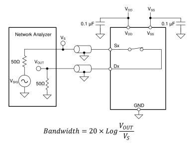
Figure 8-10. Bandwidth Measurement Setup
