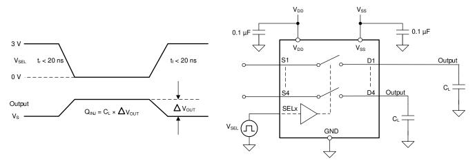
Figure 8-7. Charge-Injection Measurement Setup
