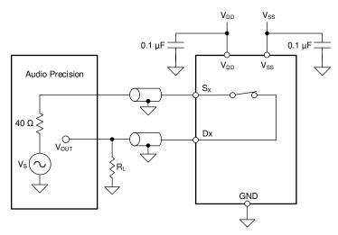
Figure 8-11. THD + N Measurement Setup
