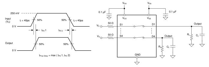
Figure 8-6. Propagation Delay Measurement Setup
