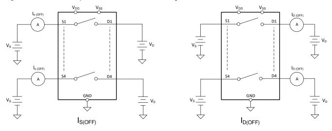
Figure 8-2. Off-Leakage Measurement Setup
