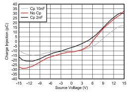
Figure 9-2. Charge Injection Compensation
