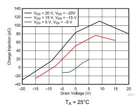
Figure 10-2. Charge Injection vs. Drain Voltage
