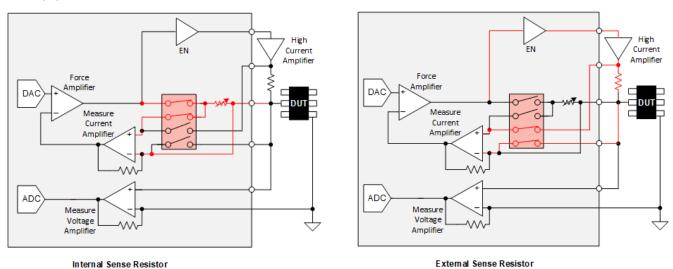
Figure 10-1. High Current Range Selection Using External Resistor
