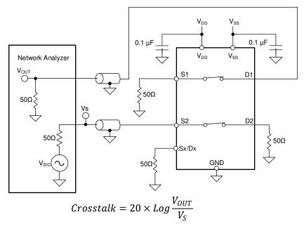
Figure 8-9. Channel-to-Channel Crosstalk Measurement Setup
