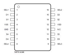
Figure 6-1. PW Package 16-Pin TSSOP Top View
