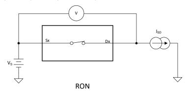
Figure 8-1. On-Resistance Measurement Setup
