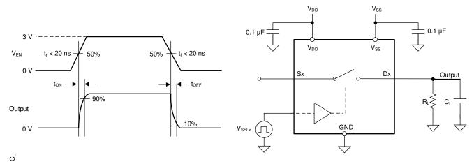
Figure 8-4. Turn-On and Turn-Off Time Measurement Setup
