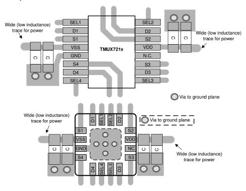
Figure 12-2. TMUX721x Layout Example
