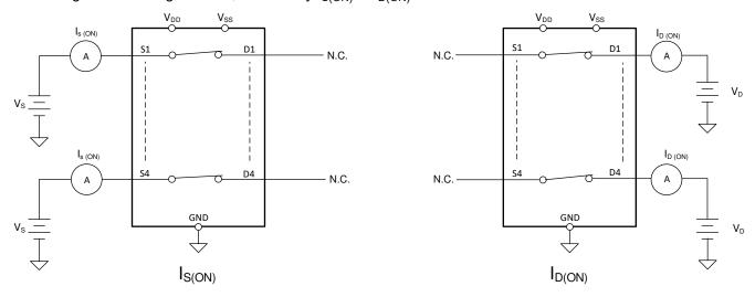
Figure 8-3. On-Leakage Measurement Setup
