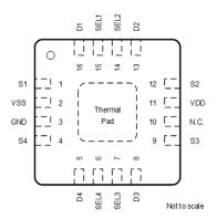
Figure 6-2. RUM Package 16-Pin WQFN Top View
