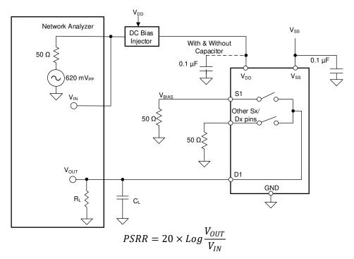
Figure 8-12. AC PSRR Measurement Setup
