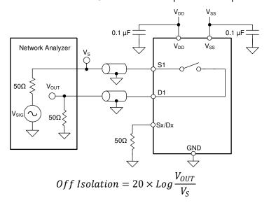
Figure 8-8. Off Isolation Measurement Setup
