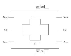
Figure 9-1. Transmission Gate Topology
