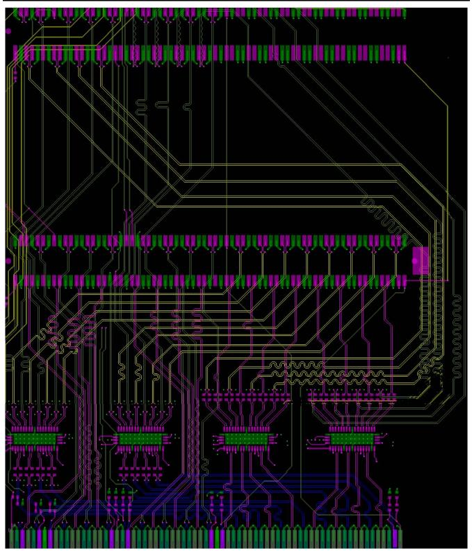
Figure 10-2. Layout example for PCIe lane muxing application
