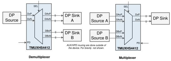
Figure 8-7. DisplayPort Main Link Demuxing/muxing
