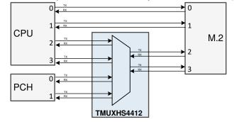
Figure 8-6. PCIe muxing to M.2 connectivitivity for hybrid SSD
