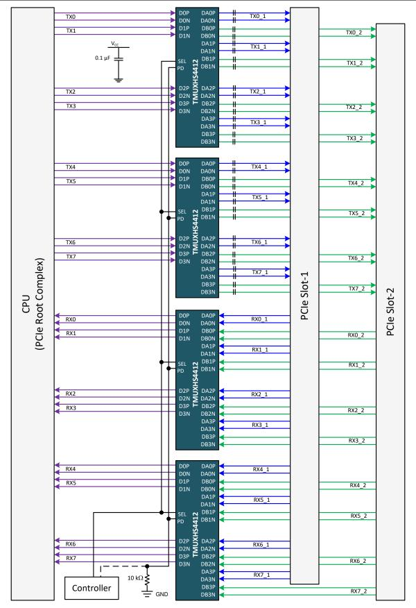
Figure 8-2. PCIe Lane Muxing
