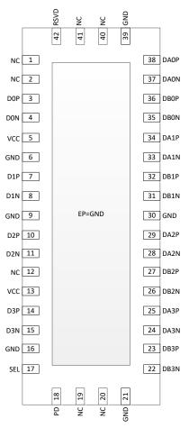
Figure 5-1. RUA package 42-Pin WQFN Top View (not to scale)
