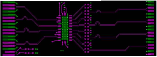
Figure 10-1. TMUXHS4412 layout example
