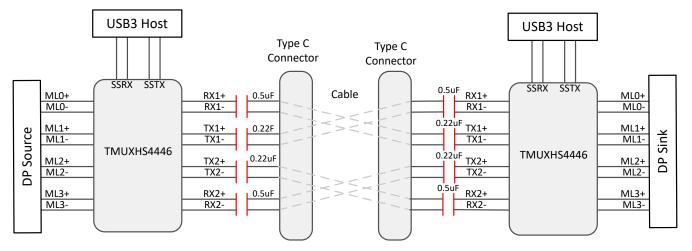
Figure 7-4. Placement of AC coupling Capacitors with Vcm > 1.8V
