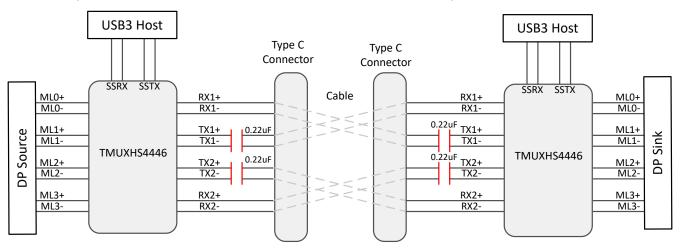
Figure 7-3. Typical Placement of AC Coupling Capacitors with Vcm ≤ 1.8V
