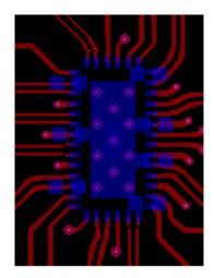
Figure 7-13. TMUXHS4446 Layout Example
