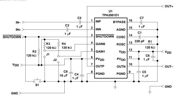
NOTE: R1, R2, and R3 are used in the EVM but are not required for normal applications.
