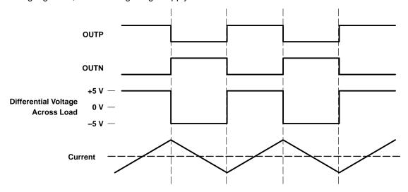
Figure 1. Traditional Class-D Modulation Scheme's Output Voltage and Current Waveforms Into an Inductive Load With No Input
