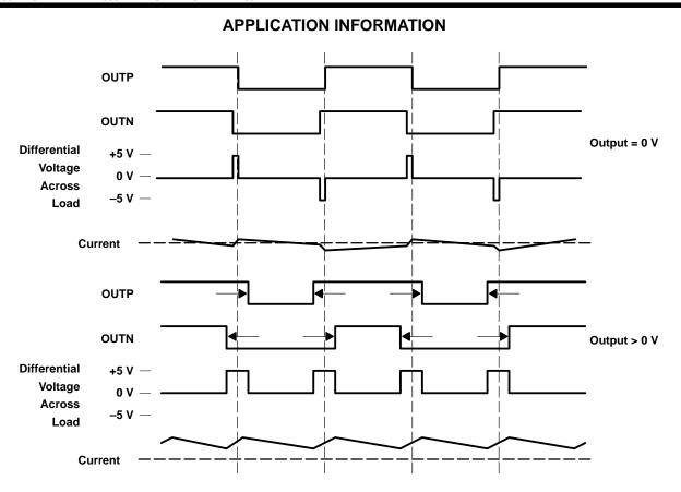
Figure 2. The TPA2001D1 Output Voltage and Current Waveforms Into an Inductive Load
