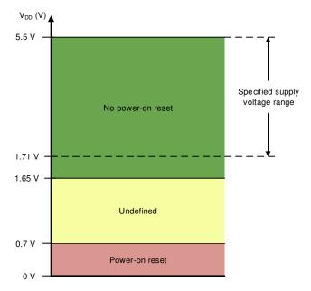
Figure 7-1. Threshold Levels for V<sub>DD</sub> POR Circuit
