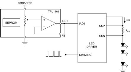
Figure 8-1. Programmable Current Limit
