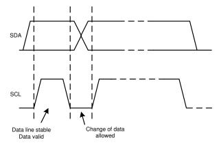
Figure 7-4. Bit Transfer on the I<sup>2</sup>C Bus
