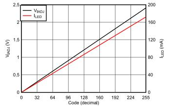
Figure 8-2. Digipot Code vs LED Current
