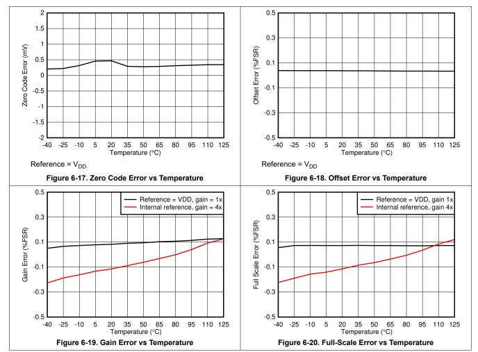
at T<sub>A</sub> = 25°C and digipot outputs unloaded (unless otherwise noted)
