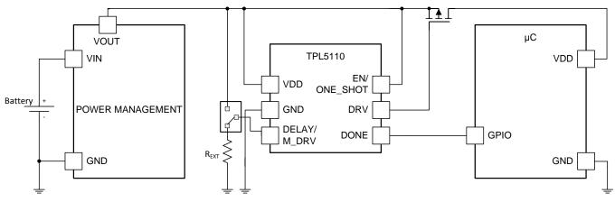
Figure 14. Manual MOSFET Power ON With SPDT Switch
