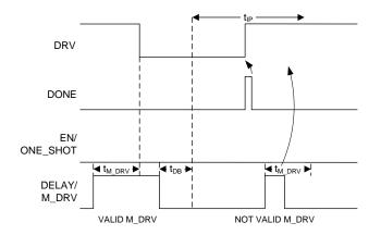
Figure 12. Manual MOSFET Power ON in One-Shot Mode
