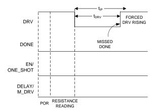
Figure 10. Start-Up One-Shot Mode (No DONE Received Within t<sub>IP</sub>)
