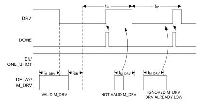
Figure 11. Manual MOSFET Power ON in Timer Mode
