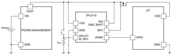
Figure 13. Manual MOSFET Power ON With SPST Switch
