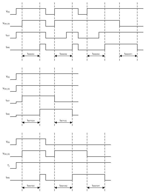
NOTES: Rise and fall times of control signals are 100 ns. Control signals include: EN, DIA\_EN, SEL1, SEL2. SEL1 and SEL2 must be set to the appropriate values.
