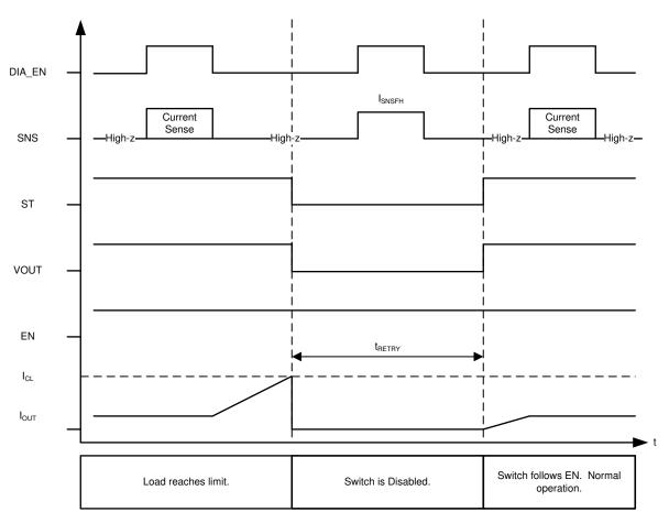
Figure 43. Current Limit – Version A,B,E - LATCH = 0
