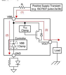
Figure 39. Current Path During Supply Voltage Transient
