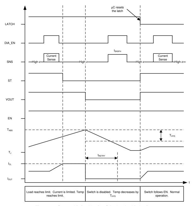
Figure 44. Current Limit - Version C,D - Latched Behavior
