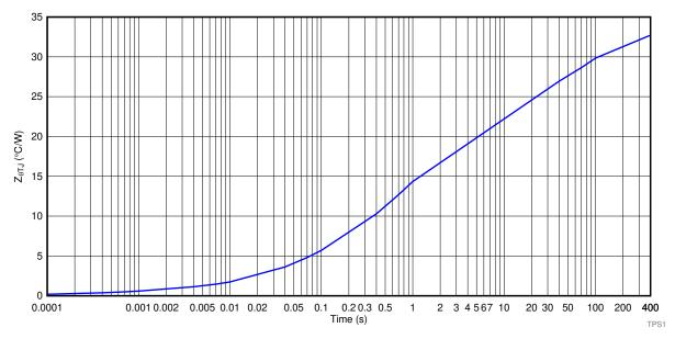
Figure 55. Transient Thermal Impedance
