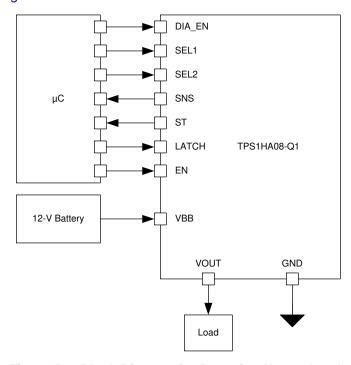
Figure 56. Block Diagram for Powering Heater Loads
