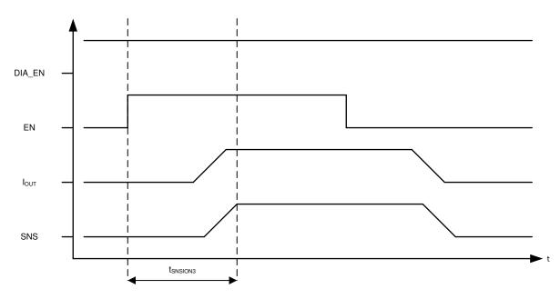
Figure 50. Current Sensing in Low-Duty Cycle Applications
