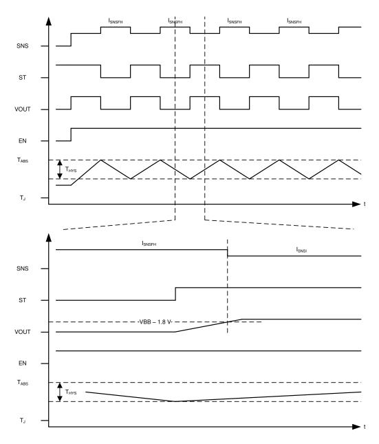
Figure 46. Fault Indication During Retry
