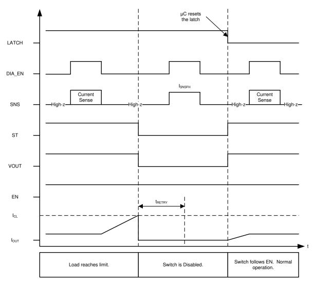
Figure 42. Current Limit – Version A,B,E - Latched Behavior
