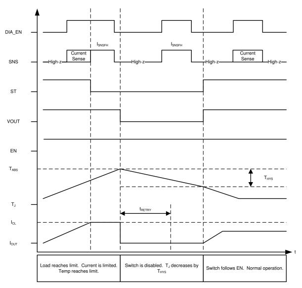
Figure 45. Current Limit - Version C,D - LATCH = 0
