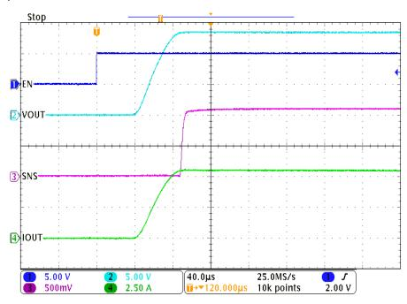
Figure 57. Heater Turn-on Time
