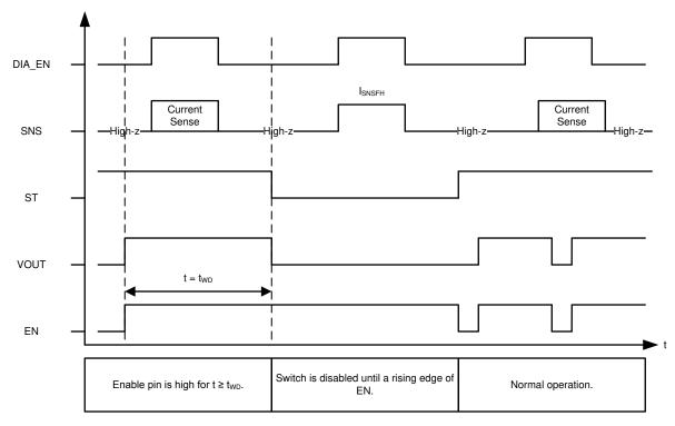
Figure 52. Enable Watchdog Timing Diagram
