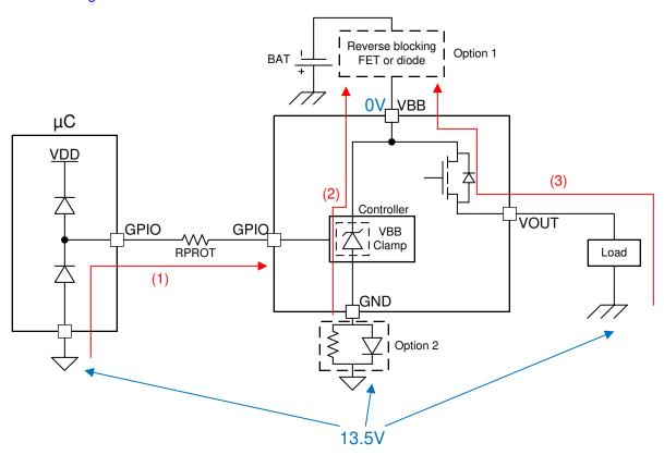
Figure 41. Current Path During Reverse Battery
