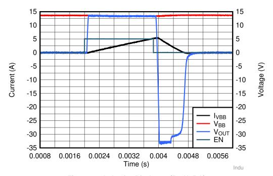
Figure 40. Inductive Discharge (5 mH, 5 A)
