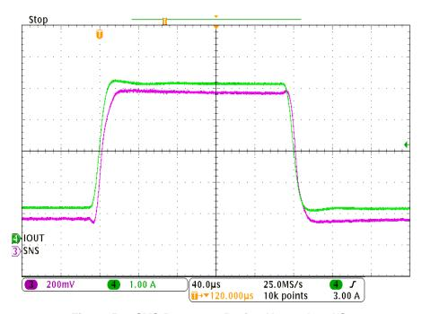
Figure 58. SNS Response During Heater Load Step
