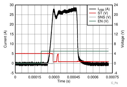
Figure 60. Overcurrent Behavior During Short Circuit Event
