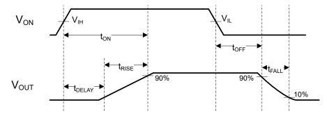
Figure 7-1.  $t_{\text{ON}}$  and  $t_{\text{OFF}}$  Waveforms
