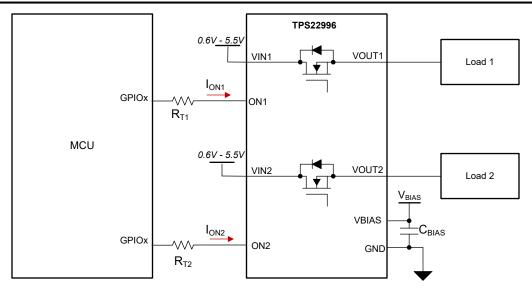
Figure 8-1. TPS22996 Adjustable Rise Time Configuration
