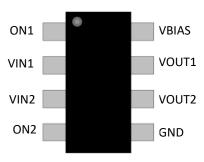
Figure 5-1. DRL Package, 8-Pin SOT (Top View)
