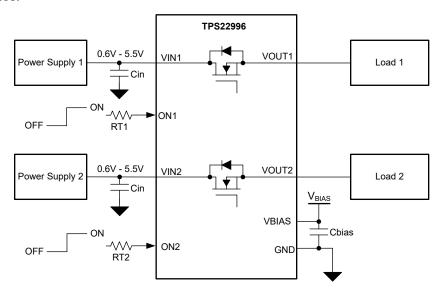
Figure 9-1. Typical Application Circuit
