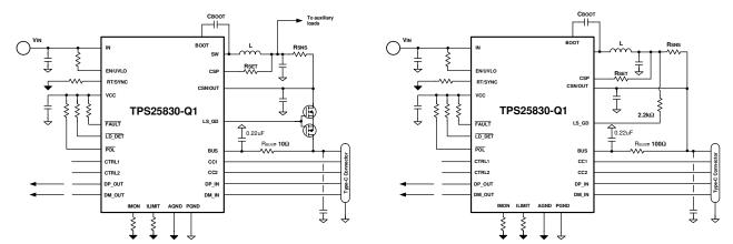
Figure 10-20. Current Limit With External MOSFET
