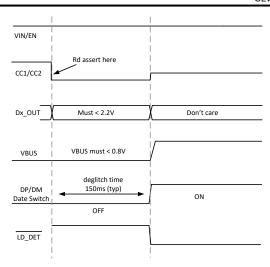
Figure 10-5. TPS25830-Q1 Pin Voltage Requirement During Rd Assert
