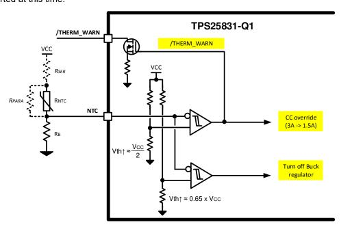
Figure 10-28. NTC Input Pin
