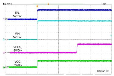
Figure 10-4. Typical Start-up Behavior,  $V_{IN}$  = 13.5 V, CC1 =  $R_d$ ,  $R_{IMON}$  = 12.6 k $\Omega$
