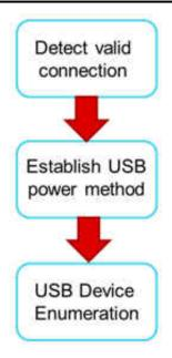
Figure 10-24. Flow of DFP to UFP Configuration
