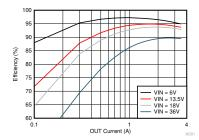
Buck Efficiency vs Output Current f<sub>sw</sub> = 400 kHz
