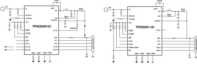
Figure 10-18. TPS25830-Q1 Buck Average Current Figure 10-19. TPS25831-Q1 Buck Average Current Limit
