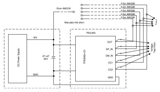
Figure 9-5. Short-to-Battery System Test Setup
