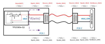
$R(wire) = R(pcb1\_VBUS) + R(conn1\_VBUS) + R(cable\_VBUS) + R(conn2\_VBUS) + R(pcb2\_VBUS) + R(USBconn\_VBUS) + R(USBconn\_GND) + R(pcb2\_GND) + R(conn2\_GND) + R(cable\_GND) + R(conn1\_GND) + R(pcb1\_GND) + R(pc01\_GND) +$
