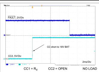
Figure 11-32. VBUS Short to BAT Recovery With External FET
