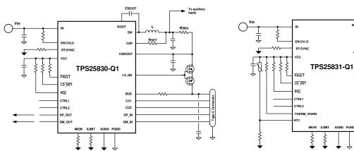
Figure 10-16. TPS25830-Q1 Current Limit with **External MOSFET**
