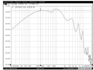
Figure 8-31. Data Transmission Characteristics vs Frequency (TPS25830-Q1)
