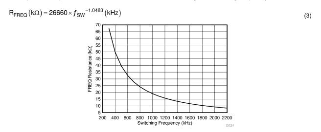
Figure 10-6. RT Set Resistor vs Switching Frequency
