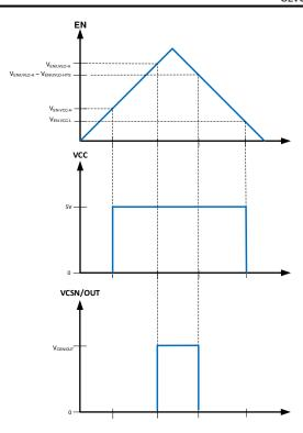
Figure 10-2. Precision Enable Behavior
