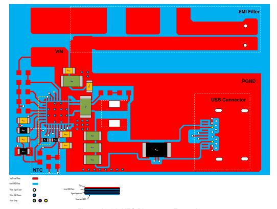
Figure 10-31. NTC Placement Example
