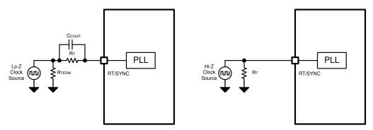
Figure 10-7. Synchronize to External Clock
