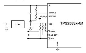
Figure 10-14. V<sub>CONN</sub> Source Using External LDO
