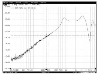
Figure 8-33. On-State Cross-Channel Isolation vs Frequency (TPS25830-Q1)
