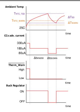
Figure 10-29. TPS25831-Q1 Behavior When Trigger NTC Threshold
