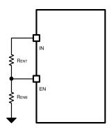
Figure 10-3. System UVLO by Enable Divider
