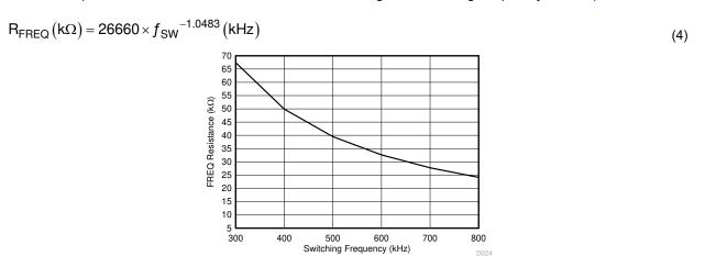
Figure 10-3. FREQ Set Resistor vs Switching Frequency
