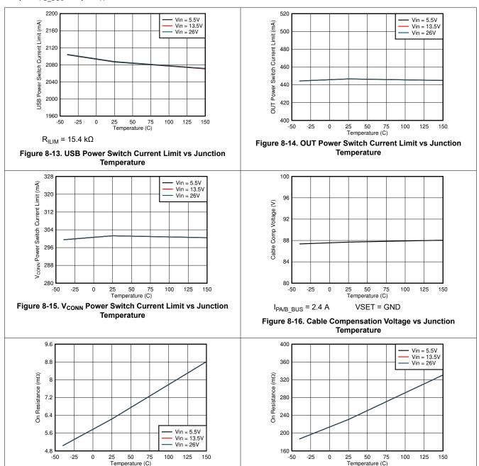
Figure 8-17. USB Power Switch On Resistance vs Junction
