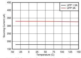
Figure 8-22. CC Sourcing Current vs Junction Temperature
