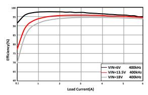
**Efficiency vs Output Current**
