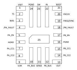
Figure 7-2. TPS25859-Q1 RPQ Package 25-Pin (QFN) Top View
