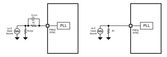
Figure 10-4. Synchronize to External Clock
