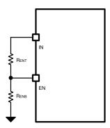
Figure 10-1. System UVLO by Enable Divider
