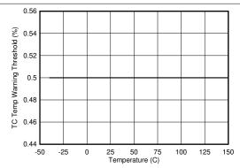
Figure 8-23. TS Temperature Wam Threshold vs Junction Temperature
