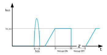
Figure 10-5. Response Time to BUS Short-Circuit
