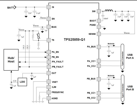
Figure 11-2. TPS25859-Q1 Typical Application Circuit for 400-kHz f<sub>SW</sub>
