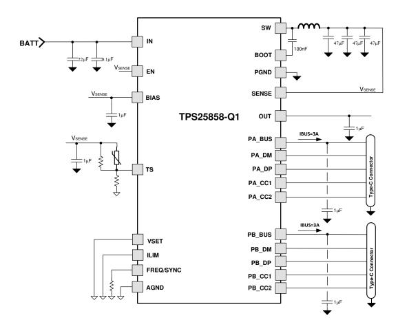
Figure 11-1. TPS25858-Q1 Typical Application Circuit for 400-kHz f<sub>SW</sub>
