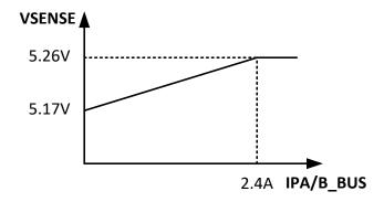
Figure 10-9. Dual Ports Cable Compensation
