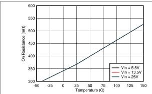
Figure 8-19. V<sub>CONN</sub> Power Switch On Resistance vs Junction Temperature
