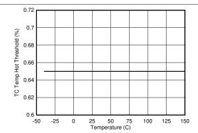
Figure 8-24. TS Temperature Hot Threshold vs Junction Temperature
