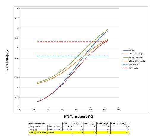
Figure 10-12. V<sub>TS</sub> Threshold Design Examples
