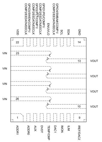
Figure 6-1. TPS25990 RQP Package 26-pin QFN Top View
