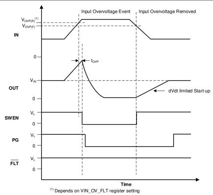
Figure 8-3. Input Overvoltage Protection Response
