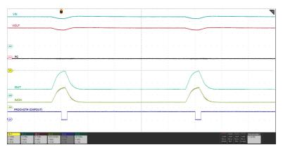
Figure 8-9. PROCHOT# Response Using Internal Comparator
