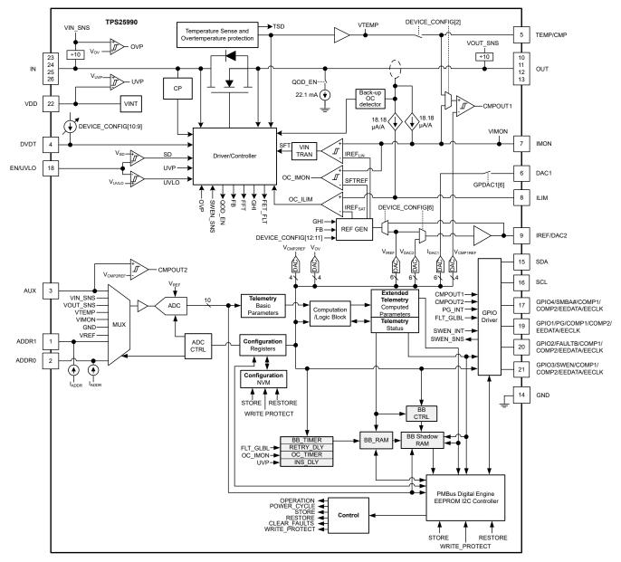
Figure 8-1. TPS25990 Functional Block Diagram
