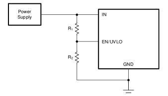
Figure 8-2. Adjustable Undervoltage Protection
