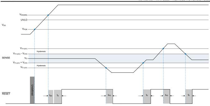
Figure 7-2. SENSE Timing Diagram
