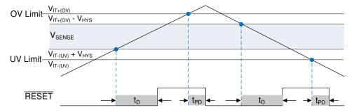
Figure 8-1. RESET output
