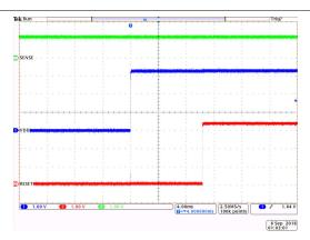
$\rm V_{DD}$  Start up from 0 V to 3.3 V,  $\rm V_{SENSE}$  = 1.2 V, CT = OPEN  $\rm V_{\overline{RESET}}$  = VDD = 3.3 V, TPS3703A4120
