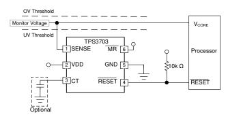
Integrated Overvoltage and Undervoltage **Detection**
