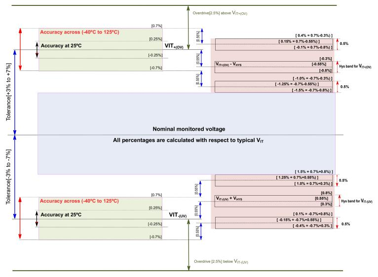
Figure 7-1. Voltage Threshold and Hysteresis Accuracy
