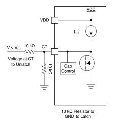
Figure 9-3. RESET Latch Circuit
