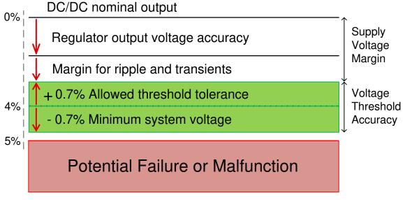
Figure 9-1. TPS3703 Voltage Threshold Accuracy
