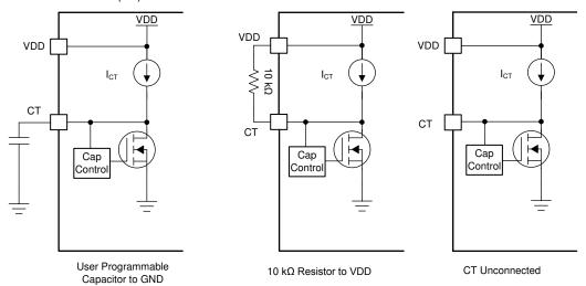
Figure 9-2. CT Charging Circuit
