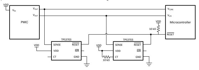
Figure 9-6. Two TPS3703 Monitoring Two Microcontroller Power Rails
