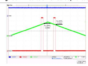
$V_{SENSE}$  ramp from 0 V to 1.4 V,  $V_{DD}$  = 3.3 V, CT = OPEN  $V_{\overline{RESET}}$  = VDD = 3.3 V, TPS3703A4120
