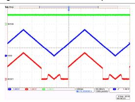
$\rm V_{DD}$  ramp from 0 V to 3.3 V,  $\rm V_{SENSE}$  = 1.2 V, CT = OPEN  $\rm V_{RESET}$  = VDD = 3.3 V,TPS3703A4120
