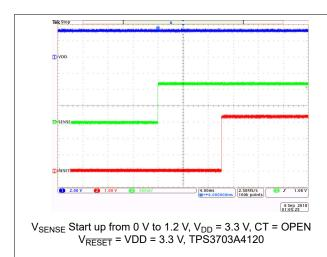
Figure 9-7. TPS3703 SENSE Start Up Function
