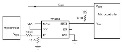
Figure 9-11. Window Voltage Monitoring with RESET Latch
