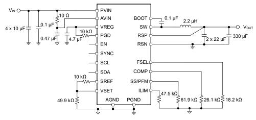
Figure 8-8. Typical Application Circuit for 5-V Output at 0.6 MHz
