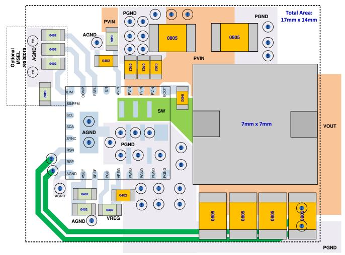
Figure 10-1. Example PCB Layout
