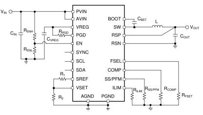
Figure 8-1. Full Analog Configuration
