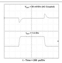
Figure 7-7. Transient Response,  $I_O$  Step 0.75 to 2.25 A.
