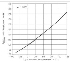
Figure 5-5. On Resistance vs. Junction Temperature
