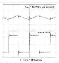
Figure 7-6. Output Voltage Ripple and PH Node, I<sub>O</sub> = 3 A
