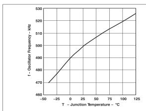
Figure 5-1. Oscillator Frequency vs. Junction Temperature
