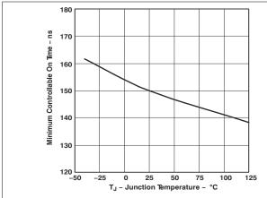
Figure 5-7. Minimum Controllable On Time vs. **Junction Temperature**
