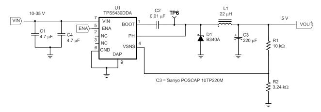
Figure 7-9. 10-V - 35-V Input to 5-V Output Application Circuit
