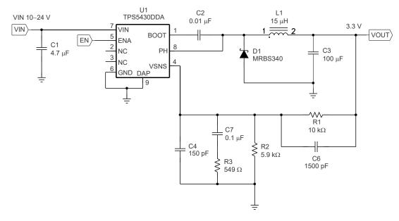
Figure 7-11. Ceramic Output Filter Capacitors Circuit
