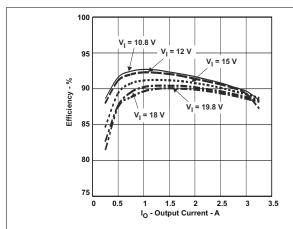
Figure 7-2. Efficiency vs. Output Current
