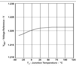
Figure 5-4. Voltage Reference vs. Junction Temperature
