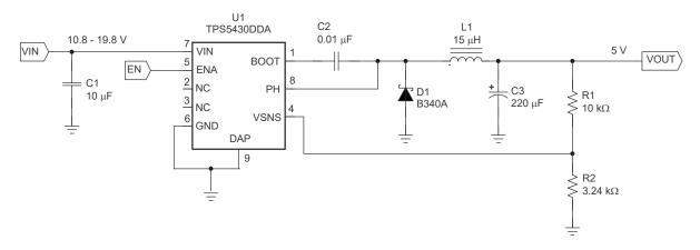
Figure 7-1. Application Circuit, 12 V Input to 5.0 V Output
