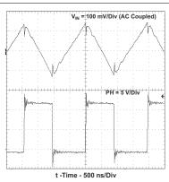
Figure 7-5. Input Voltage Ripple and PH Node,  $I_0 = 3$  A.
