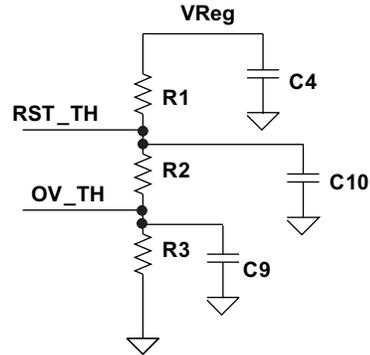
Typical cap values for RST\_TH/OV\_TH caps are between 10 pf to 100 pf range for total resistance on RSTH/OVTH divider of < 200 kΩ.
