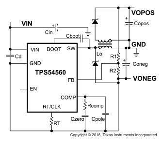
Figure 57. TPS54560 Split Rail Power Supply
