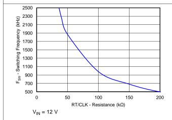
Figure 7. Switching Frequency vs RT/CLK Resistance
