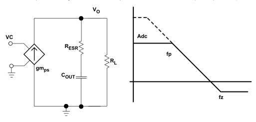
Figure 30. Simple Small Signal Model and Frequency Response for Peak Current Mode Control
