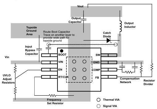
Figure 58. PCB Layout Example
