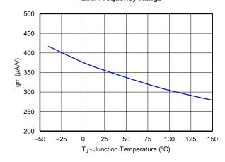
Figure 8. EA Transconductance vs Junction Temperature
