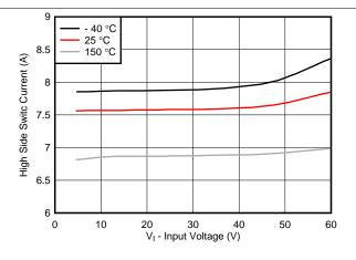
Figure 4. Switch Current Limit vs Input Voltage
