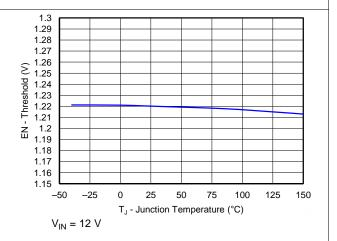
Figure 10. EN Terminal Voltage vs Junction Temperature
