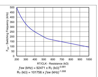
Figure 6. Switching Frequency vs RT/CLK Resistance
