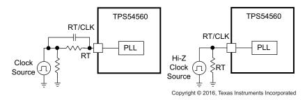
Figure 25. Synchronizing to a System Clock
