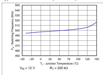
Figure 5. Switching Frequency vs Junction Temperature
