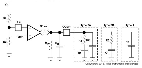
Figure 31. Types of Frequency Compensation
