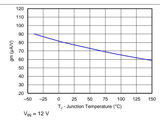
Figure 9. EA Transconductance During Soft-Start vs Junction Temperature
