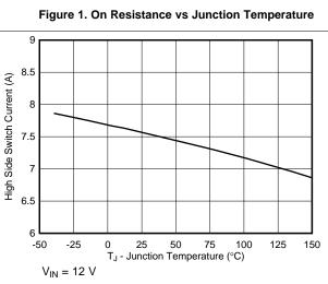
Figure 3. Switch Current Limit vs Junction Temperature
