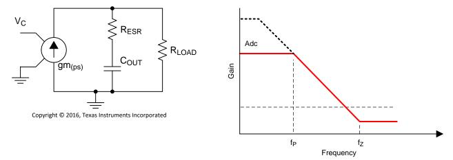
Figure 36. Small Signal Model for Peak Current Mode Control
