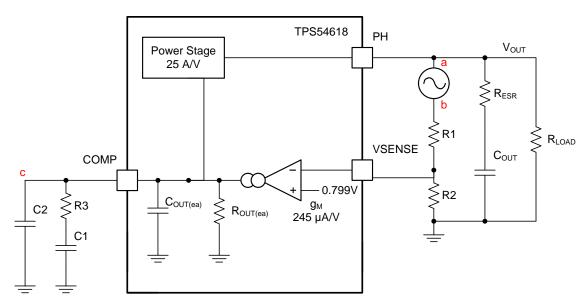
Figure 35. Small Signal Model for Loop Response
