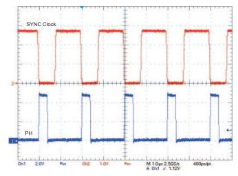
Figure 33. Synchronizing to a System Clock
