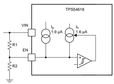
Figure 26. Adjustable Undervoltage Lockout
