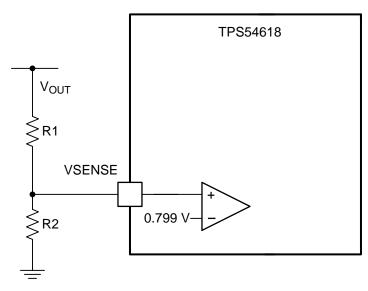
Figure 25. Voltage Divider Circuit
