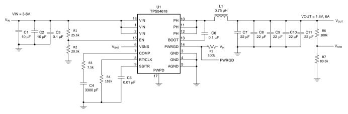
Figure 39. Typical Application Schematic TPS54618
