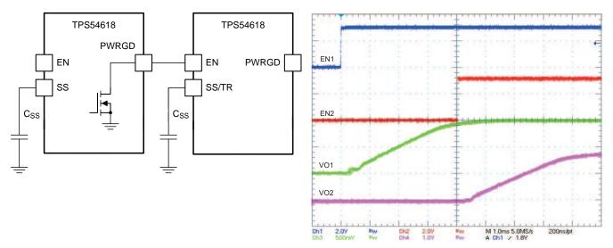
Figure 27. Sequential Start-Up Sequence
