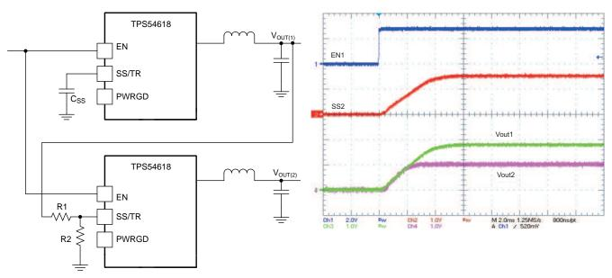
Figure 31. Ratio-Metric and Simultaneous Start-Up Sequence
