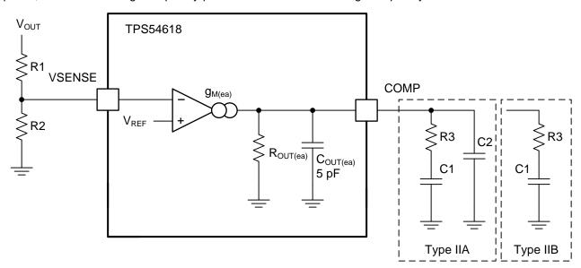
Figure 38. Types of Frequency Compensation
