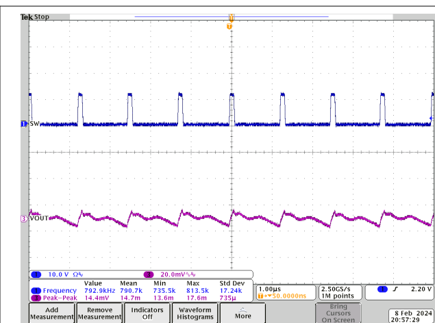
Figure 7-15. Output Voltage Ripple, 800kHz FCCM, No load, PVIN = 12V, VOUT = 1.1V
