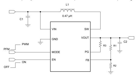
Figure 8-1. 5-V Boost Converter
