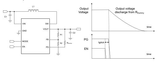
Figure 7-1. Implement Output Discharge by PG function
