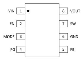
Figure 5-1. DRL Package 8-Pin SOT583 Top View
