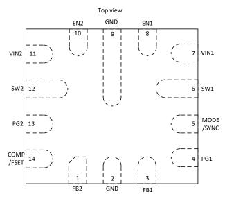
Figure 6-1. 14-Pin QFN RQR Package Top View
