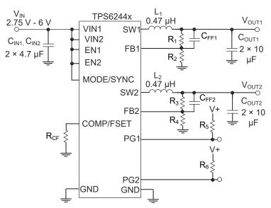
Figure 10-1. Typical Application Schematic
