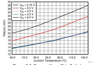
Figure 7-2.  $R_{ds(on)}$  of Low-Side Switch
