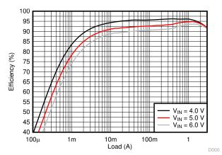
Efficiency Versus Output Current; V<sub>OUT</sub> = 3.3 V, PWM/PFM,  $f_{sw} = 2.25 \text{ MHz}$
