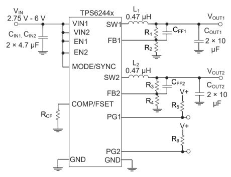
Figure 8-1. Measurement Setup
