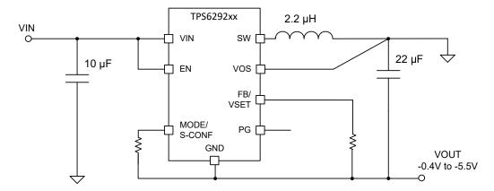
Figure 9-84. IBB Example with Internal Feedback
