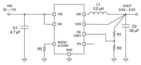
Figure 9-1. Typical Application Setup
