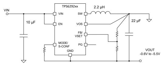
Figure 9-83. IBB Example with Adjustable Feedback
