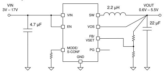
Figure 8-2. Adjustable V<sub>O</sub> Operation Schematic
