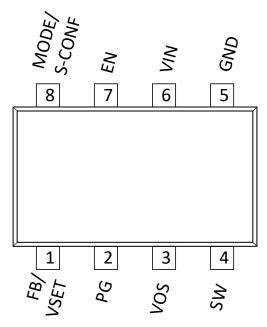
Figure 6-1. TPS629206 8-Pin DRL SOT-5X3 Pinout
