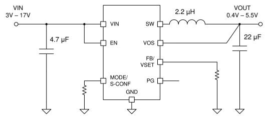
Figure 8-3. Selectable V<sub>O</sub> Operation Schematic
